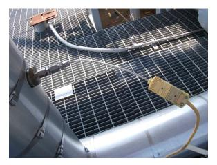
Thermocouples themselves cannot be calibrated, but the electronic amplification circuits they connect to must be routinely calibrated to ensure measurement accuracy.
