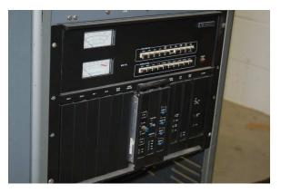
An even larger FM exciter and power amplifier unit appears in the next photograph, with a maximum rated RF power output of 22,000 Watts. This particular unit occupies the entire 19-inch wide rack frame and stands over 2 meters in height:
