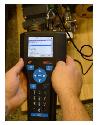
This particular HART communicator is being used to configure an electronic control module for an industrial control valve.
