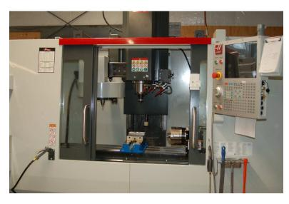
Both machines are equipped with *automatic tool-changing* capability, which means the CNC program entered into each tool is also able to instruct the machine to swap one cutting tool for another without human operator intervention. We can see a close-up of a tool "turret" here from the CNC mill:
