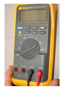
This is generally the very first piece of test equipment than an aspiring technician learns to use. Many different models exist, some with highly specialized capabilities.
