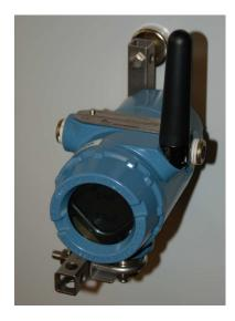
Most industrial radio systems operate in an *unlicensed* band of frequencies such as 900 MHz (in the United States) or 2.4 GHz (international) and at low power which means no FCC licenses are required to install or operate them.
