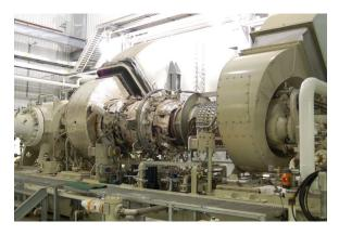
Industrial engines require substantial electronics for monitoring and control, just like modern automobile engines use electronic controls for purposes such as air/fuel ratio modulation, overtemperature detection, speed control, etc. Additionally, large industrial engines usually are equipped with exhaust emissions monitoring, vibration monitoring, and other controls not typically seen on automobiles.
