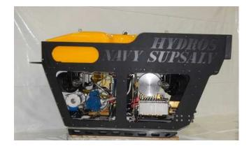
Such vehicles contain on-board propulsion systems, sonar navigation aids, magnetic compass, manipulator arms, and connect to a surface ship using an umbilical cable that often uses optical fibers for noise-free data communications.
