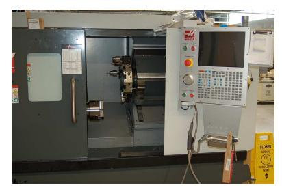
Inside the compartment where the machining takes place, the shiny object on the left (called a *chuck*) securely grips the part being turned, while tools held in the rotatable "turret" may be brought into contact with the rotating part to shape it.
