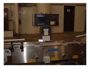
Closely related to scales are devices called *weighfeeders*, which combine scales with a moving conveyor belt used to measure the flow rate of solid powder or granular materials. Here we see a weighfeeder used to control the feed rate of caustic soda ash into water at a drinking water treatment plant, along with its electronic display screen showing the status of soda ash powder flow:
