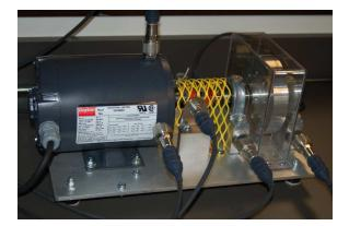
This apparatus is for demonstration purposes only, but show the ways in which vibration probes are typically installed on a large rotating machine.
