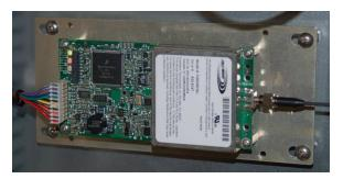
Another form industrial radio communications often takes is radio transceivers built directly into the field device, rather than as an interface between some field device and a central host. Consider the following example of a *temperature transmitter* which receives an electrical input from a temperature sensor such as a thermocouple or an RTD and broadcasts the temperature data via its black-colored antenna:
