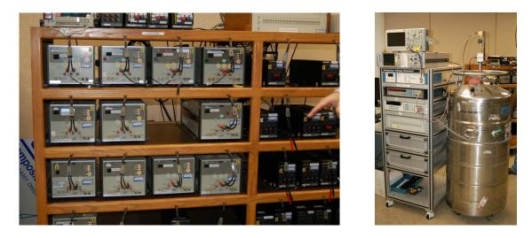
Virtually all industries require accurate measurement, and standards laboratories are the places where calibration equipment gets checked. This process of comparing calibrations against standards of higher quality, all the way up to primary standards laboratories, is called *traceability*. Like pedigree for animal breeding, traceability documents the integrity of the "calibration chain" extending back to those primary standards.
