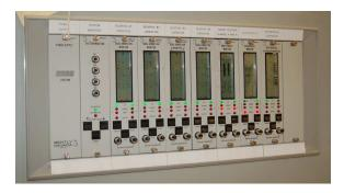
A more modern example of a vibration monitoring system is this "rack" chassis with plug-in cards housing individual electronic circuits for sensor signal conditioning, processing, power supplies, digital communication, etc.:
