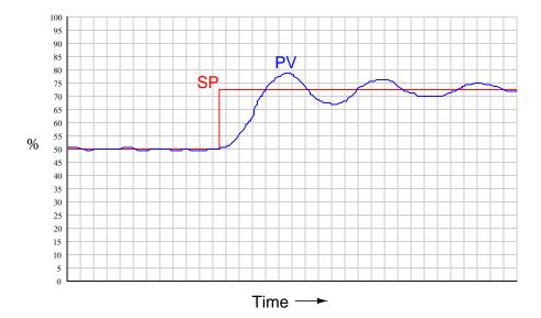
If the gain is set too low, the process response will be stable under steady-state conditions but relatively slow to respond to changes in setpoint, as shown in the following trend recording:
