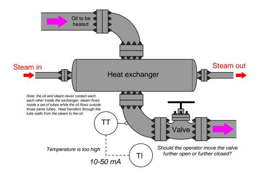
In any automated (controlled) system, there is a process variable, a setpoint, and a manipulated variable. There is also something called a load, which influences how well the control system is able to maintain setpoint. Provide a general description for a "load," and then identify the load(s) in each of the these processes.
