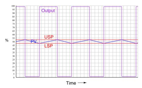
As you can see, the degree of control is rather poor. The process variable "cycles" between the upper and lower setpoints (USP and LSP) without ever stabilizing at the setpoint, because that
