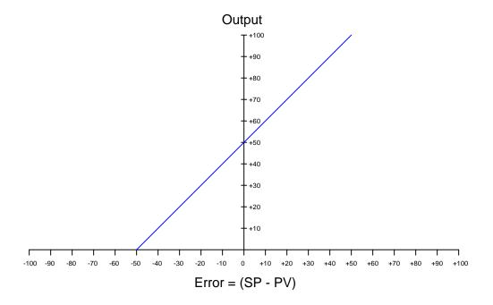
In this graph the bias value is 50% and the gain of the controller is 1. Changing the bias value (b) of the controller shifts the line up or down. Changing the gain value  $(K_p)$  alters the slope of the line for more or less aggressive control action.
