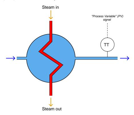
The signal output by the transmitter (represented by the "PV" dashed line), representing the heated fluid's exiting temperature, is called the *process variable*. Like a variable in a mathematical equation that represents some story-problem quantity, this signal represents the measured quantity we wish to control in the process.
