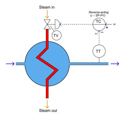
Here, the circle with the letters "TC" in the center represents the controller. Those letters stand for Temperature Controller, since the process variable being controlled is the process fluid's *temperature*. Usually, the controller consists of a computer making automatic decisions to open and close the valve as necessary to stabilize the process variable at some predetermined *setpoint*.
