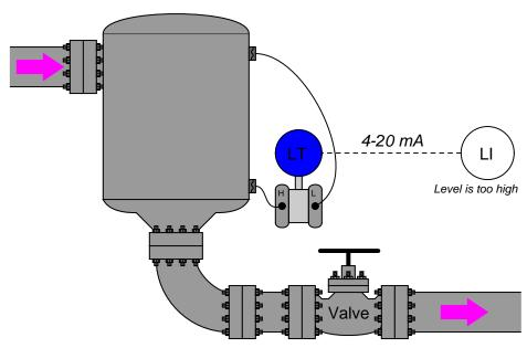
Should the operator move the valve further open or further closed?
