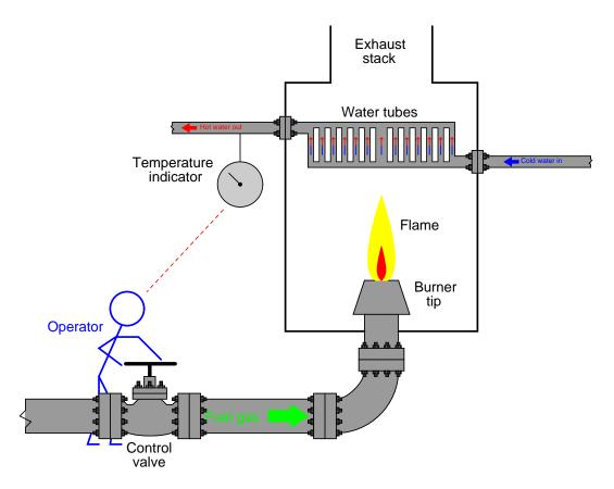
Does the operator play the part of a *diect-acting* controller, or a *reverse-acting* controller, in this process control scenario?
