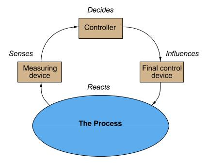
One of the basic diagnostic strategies for any instrumentation system is to assess whether the  $input\ value(s)$  and  $output\ value(s)$  correspond for each instrument. We may apply this same strategy to each of the four elements of a feedback control "loop" to identify where the problem might exist. If you encounter one of these four system portions whose output does not correspond with its input, you know that portion of the system is faulted.
