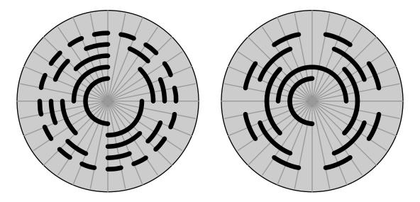
Assuming that the darkest areas on the illustration represent slots cut through the disk, and the grey areas represent parts of the disk that are opaque, mark the "zero," "one," and "two" sectors on each disk.
