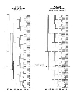
The electron beam's periodic sweep crosses the face of the mask in the horizontal axis (as the masks are shown above), so that the beam "probes" one row at a time. The vertical position of the beam on the mask is determined by the sampled analog signal. Each column of holes on the mask represents one bit (one "digit" as described by Gray) in the binary word. For the sample masks shown, a seven-bit binary sequence is generated for every sweep of the beam from left to right. For an
