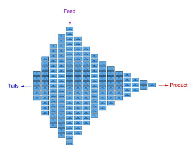
The sheer number of gas centrifuges employed at a large-scale uranium enrichment facility is impressive. At the Natanz facility, where just one cascade contained 164 centrifuges, cascades were paralleled together in *sub-units* of six cascades each (984 centrifuges per sub-unit), and three of these sub-units made one cascade *unit* (2952 centrifuges total).
