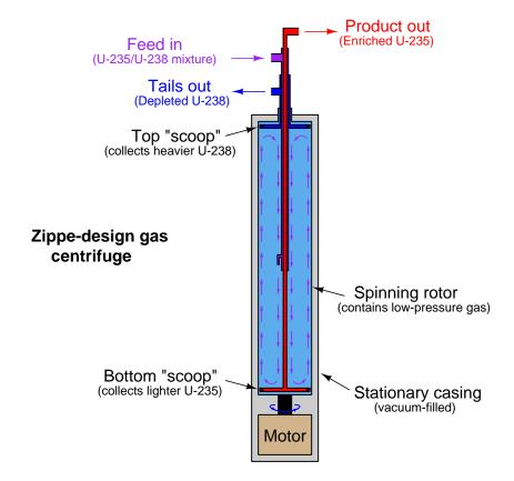
Like the separation membranes used in gaseous diffusion processes, each gas centrifuge is only able to enrich the UF<sup>6</sup> gas by a very slight amount. The modest enrichment factor of each centrifuge necessitates many be connected in series, with each successive centrifuge taking in the out-flow of the previous centrifuge in order to achieve any practical degree of enrichment. Furthermore, gas
