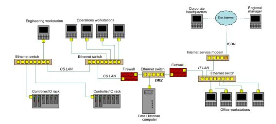
For each firewall at the boundary of the DMZ, its respective ACL must be configured so as to only permit ("whitelist") the Data Historian computer, which is the "server" device within the DMZ. The purpose of a Data Historian is to poll process data from the control system at regular intervals, store that data on a high-capacity data drive, and provide that data (i.e. "serve the data") to external computers<sup>7</sup> requesting it.
