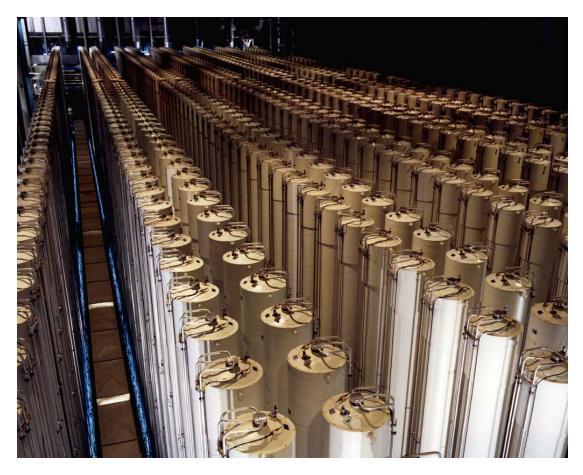
Without any familiar objects in this photograph it is difficult to get an accurate sense of physical scale, but know that each of these centrifuge units measures 40 feet in height.
