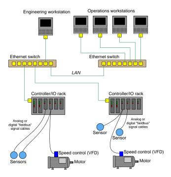
It would be wise to configure the PC workstations with password authentication to ensure only authorized personnel have access to the functions of each. The engineering workstation in particular
