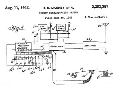
The oscillator's pattern of frequency-changes is controlled by a paper tape moved between two spools, with holes punched in the tape in a manner not unlike that of a player-piano mechanism which served as this invention's inspiration. Although "frequency-hopping" radio communication technology may be used for many purposes, these inventors intended it for the remote guidance of torpedoes to be used by the Allied forces during World War Two. In the inventors' own words:
