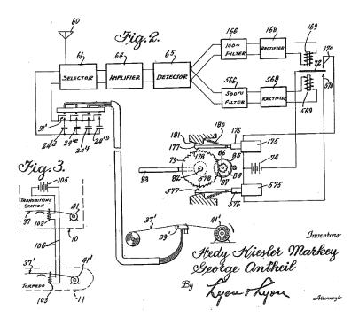
An interesting feature of this design is that the transmitter was capable of "hopping" between more frequencies than the receiver was built to receive, and this was done purposely to permit the occasional broadcast of false signals which would further confound any attempt for an enemy to intercept or jam the radio transmissions:
