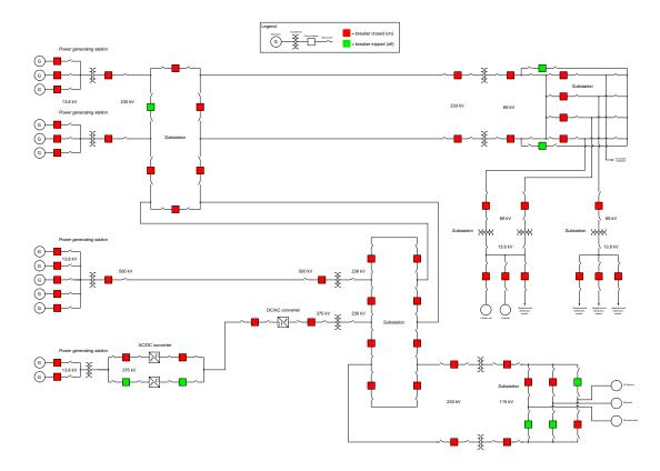
Identify any "high-value targets" for cyber-attack in this system. These would be components in the power system most likely to result in extended outages and/or maximum effect from an outage of any duration.
