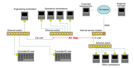
The air gap between the two Ethernet-based networks not only preclude any direct data transfer between one and the other, but also ensure their respective data traffic never collides. This simple design should be used whenever possible, as it is simple and effective on multiple fronts.
