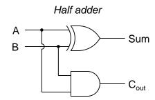
This circuit is known as a *half adder* because it is incomplete: it is able to generate a carry bit, but it cannot *receive* a carry bit from another adder circuit which is important if we wish to gang multiple adders together so as to be able to add more than just two bits together.
