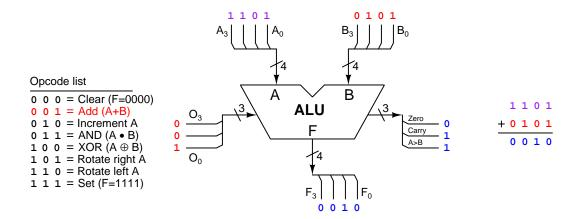
We must ignore the carry status flag since we are using signed 4-bit integers, which means a fifth bit has no meaning. The result is simply 0010 which of course is a positive two.
