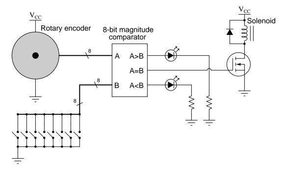
Identify specific component failures that could result in the solenoid coil not energizing in this condition.
