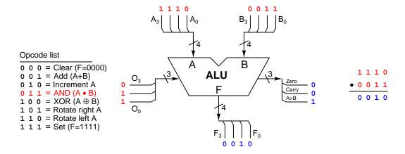
Recall from the truth table of an AND function that any 0 input to an AND function guarantees a 0 output. Thus, by ANDing one digital word with another we prioritize all 0 bit states, so that the result contains every 0 bit contained in both words. The only way a 1 bit can exist in the result is if both words contained 1 bits in that same position.
