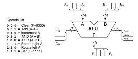
This ALU offers eight unique operations, each one specified by a three-bit opcode. Each operation acts upon either one or two four-bit operands, A by itself or A combined somehow with B. We may represent the operand and result circuitry of this ALU in terms of logic gates and multiplexers:
