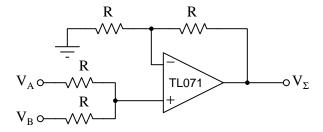
These two circuits perform the same mathematical function, yet the manners in which they perform this function are quite different. Compare and contrast the digital adder and the analog summer circuits shown here, citing any advantages or disadvantages of each.
