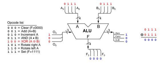
The operands' equality is indicated by the ALU's Zero status flag terminal outputting a 1 state following the XOR operation. Contrast this with a scenario where the two operands are unequal:
