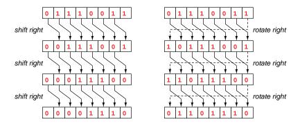
With enough shift operations, the original word's bits become entirely replaced by 0's. However, rotate operations merely circulate the bit-states and never replace them with 0's.
