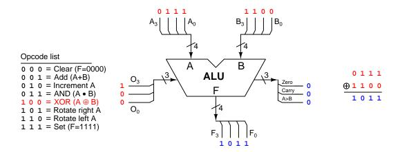
Here, we have successfully inverted the left-two bits of operand A, turning 0111 into 1011.
