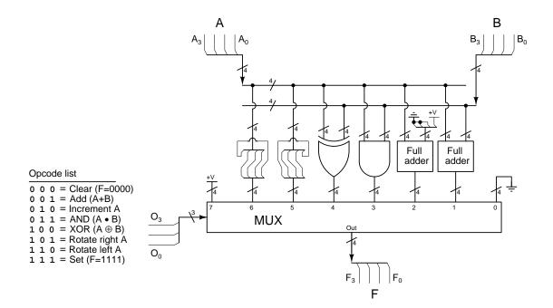
Real ALUs are not designed quite like this, because it would require more transistors than absolutely necessary. However, the concept of having individual functions (e.g. full adder, AND,
