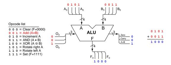
The actual process of addition highlighted on the right-hand side of the diagram is as easy as it looks: simply apply the same technique you learned for adding multi-digit decimal numbers, and you will get the same result shown here. Note the A>B status flag bit that is set simply by virtue of the fact operand A is larger than operand B.
