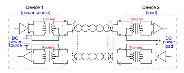
Explain what function(s) the transformers provide in this system, and how they allow DC power to travel through the wire pairs from source to load without interfering with the Ethernet data signals, which are AC.
