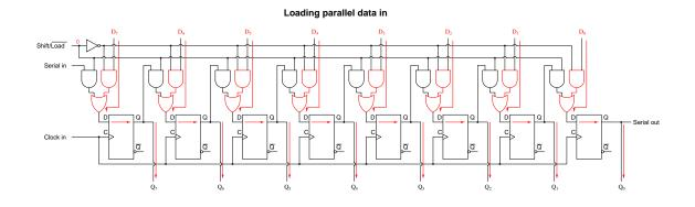
In the "Shift" mode of operation these steering gates route data from one flip-flop stage to the next as shown in red below:
