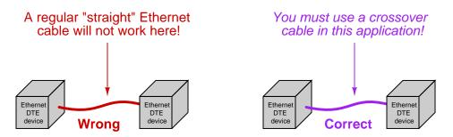
Furthermore, the same problem exists when multiple hubs are connected to form larger networks. Since each hub is a DCE device, a straight-through cable connecting two hubs together will pass transmitted signals from one hub directly to the "transmit" pins of the other hub, not the "receive" pins as it needs to. Consequently, a "crossover" cable should be used to connect two Ethernet hubs together in order to avoid this problem:
