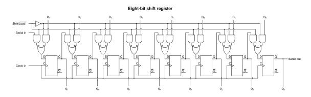
The AND/OR gate networks *steer* digital data to those flip-flops from different sources. In the "Load" mode of operation these steering gates route data from the parallel input terminals to the eight flip-flops as shown in red below:
