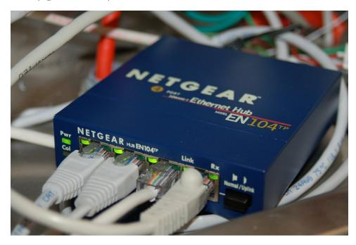
Note the LED indicator lights by each port on the hub. One LED indicates whether or not the cable is active (when a powered Ethernet DTE device is plugged into that port of the hub), while the other LED indicates traffic on the cable (by blinking). These LEDs are very helpful for identifying a crossover problem. This hub even has an LED indicating the occurrence of collisions (the "Col" LED just below the main power LED), giving simple visual indication of collision frequency.
