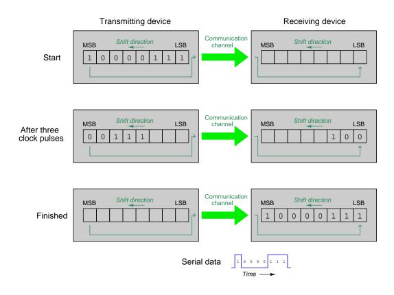
Shift registers are comprised of *flip-flops*, and are designed to move bits of data along from one flip-flop to another in sequence at the command of the clock pulse signal. The action of a shift register may be likened to a conveyor belt where packages move on to and off of the belt in various ways as shown below, the packages representing bits and the conveyor's motion representing the clock pulse:
