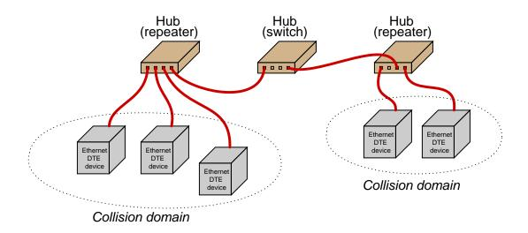
Of course, collisions between these two domains may still occur, for instance if a device in the first domain tries to transmit to a device in the second domain at the exact same time that a device in the second domain attempts to transmit to a device in the first.
