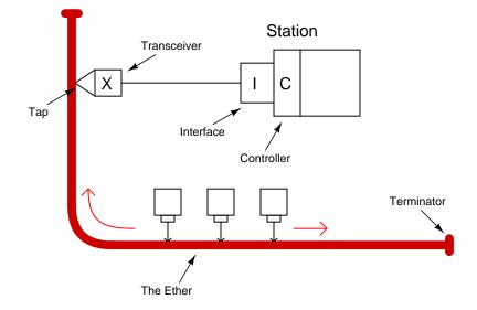
Explain the basic concept behind Metcalfe's Ethernet system, and why he chose the word "ether" to name it. Also, identify the bit rate (speed) at which his original Ethernet communicated at.
