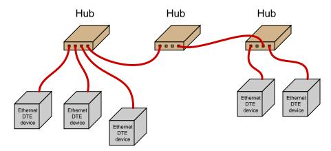
Repeating hubs may be connected together to form larger networks<sup>2</sup>:
