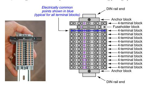
Screwless terminal blocks (using internal spring clips to clamp wire and component lead ends) are preferred over screw-based terminal blocks, as they reduce assembly and disassembly time, and also minimize repetitive wrist stress from twisting screwdrivers. Some screwless terminal blocks require the use of a special tool to release the spring clip, while others provide buttons<sup>9</sup> for this task which may be pressed using the tip of any suitable tool.
