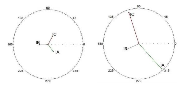
First, identify the phase rotation of this power system based on the color-coding of the phasors. Is it ABC or is it CBA? How are you able to determine this fact.
