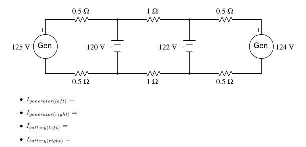
Next, write a computer program in a text-based language (e.g. C, C++, Python) that will calculate all the same currents given fixed resistance values and user-input voltage values.
