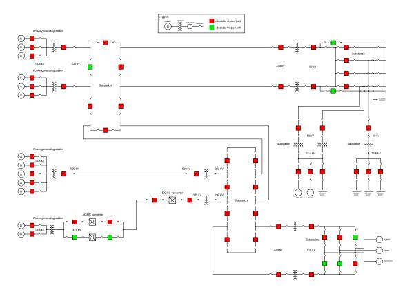
An example of a modern power grid is shown in the following *single-line diagram*<sup>1</sup>:
