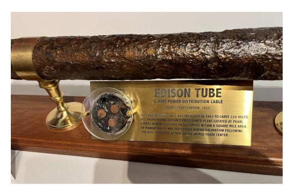
A cross-section of this cable shows the three copper conductors encased in tar within the metallic sheathing of the cable. Despite the obvious corrosion evident on the outside of the cable, it is clear that the copper conductors themselves are well-preserved.
