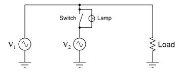
Imagine a condition where generator  $V_1$  is operating and powering the load, but generator  $V_2$  is stopped with its disconnecting switch in the open position. In this condition the lamp will glow steadily, operating on the difference of potential between the power line (full AC voltage) and the idle generator  $V_2$  (0 Volts).
