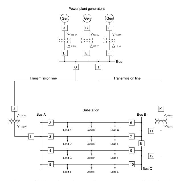
Suppose Load F fails in such a way that it draws far more current than it should. Identify which circuit breaker(s) must trip in order to interrupt the fault current while maintaining power to as many other loads as possible.
