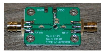
Amplification is provided by the black-colored integrated circuit (IC) in the center of the board, with DC power entering at the top. Note the two decoupling capacitors soldered between the  $V_{CC}$  trace and the ground plane. Note also the coupling capacitors on both the input and output traces to prevent the amplifier IC from seeing DC in the incoming signal or to output DC to the outgoing SMA connector.
