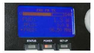
The power amplifier takes the exciter's signal and boosts its power to 7.6 kW, with only 21 Watts of reflected power coming back from the antennas. Normally the power output is 17 kW, but was turned down for this photographic opportunity to limit RF exposure while in the transmitter shack:
