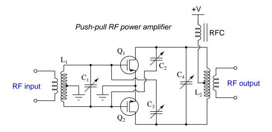
Tank circuit  $C_1/L_1$  tunes the input of the amplifier while  $C_4/L_2$  tunes the output and helps to suppress unwanted harmonics (especially when operated in class B or class C modes). Capacitors  $C_2$  and  $C_3$  serve to neutralize the amplifier, helping to prevent self-oscillation. Note how the input signal for this amplifier happens to be balanced as well (i.e. two un-grounded terminals).
