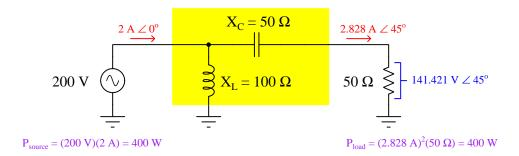
One way to view these LC impedance-transformation networks conceptually is to view the series-connected component (with the load) as adding to the load's impedance, and the parallel-connected component (with the source) correcting that increased impedance to become purely resistive as seen by the source.
