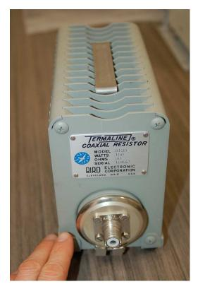
One should *never* operate an RF power amplifier without a suitable load connected to its output, whether that be a proper antenna or a "dummy" load of proper resistance. Failure to do so may actually cause damage to the amplifier's internal circuitry! Even Citizen's Band (CB) radio transceivers rated at just 5 Watts of output power come with warnings not to transmit without the output connected to a proper load.
