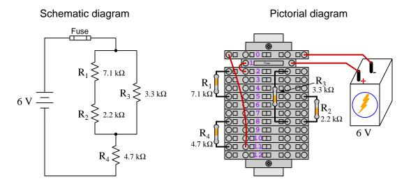
Numbering on the terminal blocks provides a very natural translation to SPICE<sup>10</sup> netlists, where component connections are identified by terminal number:
