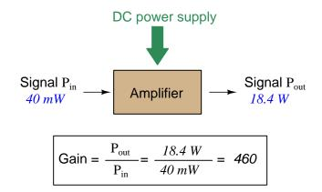
An alternative way to express the gain of this amplifier is to do so using the unit of the *Bel*, defined as the common logarithm of the gain ratio:
