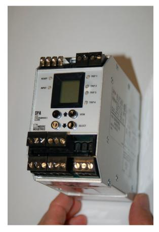
In addition to providing alarm capability, this SPA module also provides a digital display (a small LCD screen) to show the analog signal value for operational or diagnostic purposes.
