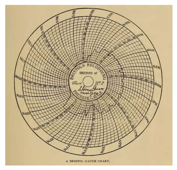
This particular recording is of a steam boiler's pressure over a 24-hour period, showing pressure build-up beginning at 4:00 AM and boiler shut-down at 9:30 PM. This steam boiler's pressure appears to have been operated at approximately 70 PSI. Dips and peaks in the trace reflect changes in steam demand as well as irregularities in the firing of the boiler's coal furnace.
