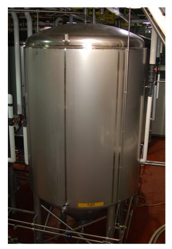
If the beer becomes too warm, the controller sends an increased signal to the glycol valve sending more chilled glycol through the vessel's jacket to remove heat from the beer. Since the relationship between the controller's process variable and its output is direct (i.e. rising PV results in rising Output), the controller needs to be configured for direct action.
