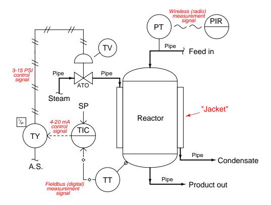
The purpose of this control system is to ensure the chemical solution inside the reactor vessel is maintained at a constant temperature. A steam-heated "jacket" envelops the reactor vessel, transferring heat from the steam into the chemical solution inside. The control system maintains a constant temperature by measuring the temperature of the reactor vessel, and throttling steam from a boiler to the steam jacket to add more or less heat as needed.
