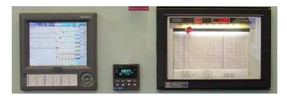
on the top which presumably rings under alarm conditions. Regarding the strip chart record, note the "compressed" scale, whereby successive divisions of the vertical scale become closer in spacing, reflecting some inherent nonlinearity of the pressure-sensing mechanism.
