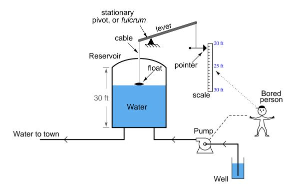
As crude as it is, this system contains *instrumentation*, and we may apply standard instrumentation terms to its components. Apply the following terms to this water-supply system, as best as you can:
