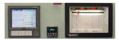
on the top which presumably rings under alarm conditions. Regarding the strip chart record, note the "compressed" scale, whereby successive divisions of the vertical scale become closer in spacing, reflecting some inherent nonlinearity of the pressure-sensing mechanism.
