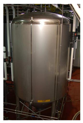
If the beer becomes too warm, the controller sends an increased signal to the glycol valve sending more chilled glycol through the vessel's jacket to remove heat from the beer. Since the relationship between the controller's process variable and its output is direct (i.e. rising PV results in rising Output), the controller needs to be configured for direct action.
