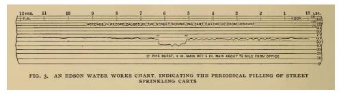
Several interesting details<sup>1</sup> may be seen on this particular recording, including pressure fluctuations caused by periodic draws of water from a fire hydrant to fill street carts used to spray
