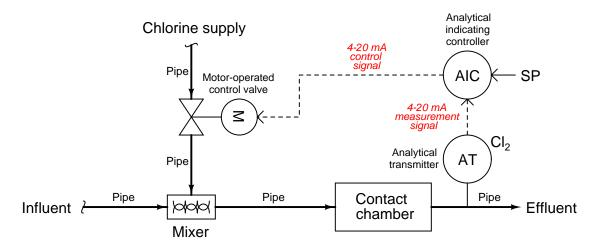
Chlorine gas coming through the control valve mixes with the incoming water (influent), then has time to disinfect in the contact chamber before exiting out to the environment.
