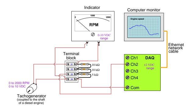
Suppose the diesel engine happens to be running at full speed (2000 revolutions per minute, or 2000 RPM). Identify the amount of voltage we would expect to measure between the following pairs of points in the circuit at this engine speed:
