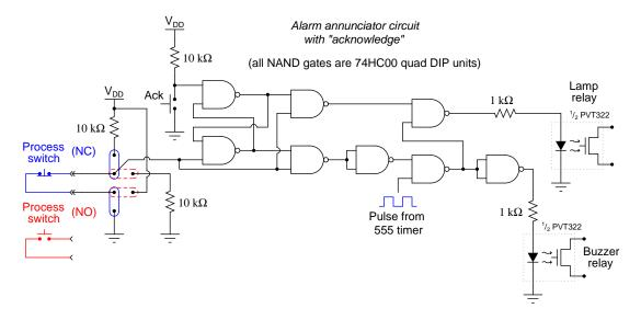
Note the jumper options shown in the diagram: one set of jumper positions configures the alarm for a process switch that alarms when its contacts open, and the other positions configures the alarm for a process switch that alarms when its contacts close. In either case, the circuit is designed to indicate an alarm status when the line going in to the lower-left NAND gate goes *high*.
