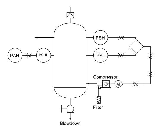
The "PSH" (pressure switch, high) activates when the air pressure inside the vessel reaches its high control point. The "PSL" (pressure switch, low) activates when the air pressure inside the vessel drops down to its low control point. Both switches feed discrete (on/off) electrical signals to a logic control device (symbolized by the diamond) which then controls the starting and stopping of the electric motor-driven air compressor.
