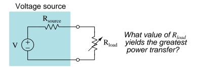
As a first step in answering this question, let us consider a real voltage source powering a short versus powering an open. From these two "thought experiments" we should be able to plot a path forward to a general answer:
