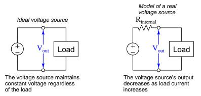
The closer to ideal a voltage source is, the less its internal resistance. An ideal voltage source is considered to have zero internal resistance.
