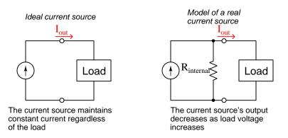
The closer to ideal a current source is, the more its internal resistance. An ideal current source is considered to have infinite internal resistance.
