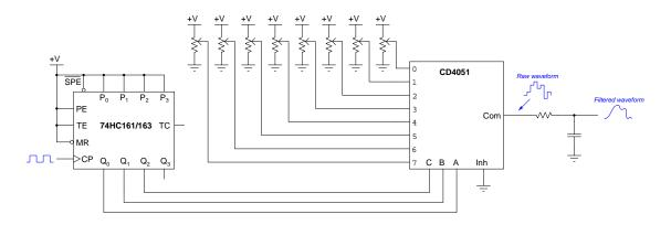
The clock signal may be supplied by a benchtop signal generator, by the output terminal of a 555 timer IC connected for astable operation, or any other suitable digital pulse signal source. Since the mux cycles through all its channels every *eight* counts of the counter IC, the final output signal will have a frequency one-eighth that of the digital clock pulse driving the counter.
