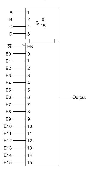
Show the wire connections necessary to make the multiplexer output the specified logic states in response to the data select (A, B, C, and D) inputs.
