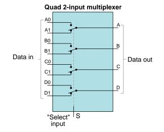
These multiplexers find popular use selecting between one of two four-bit digital *words*, in this case word 0 and word 1. Demultiplexers with similar formats also exist, directing a digital word to one of two banks of output lines.
