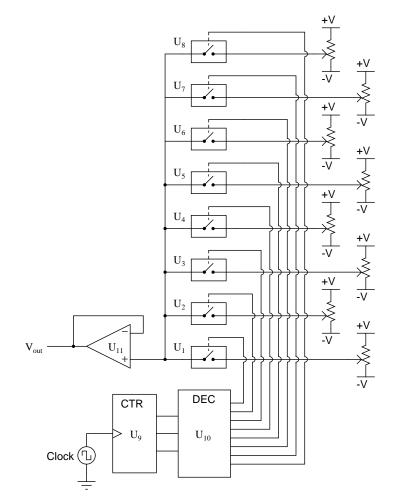
Explain what effect a *shorted* bilateral switch would have on the output waveform. Be as specific as possible.
