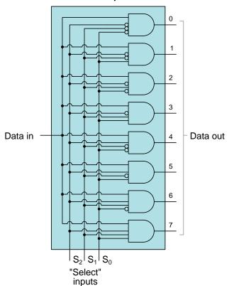
Interestingly, a demultiplexer is identical to a *binary decoder* equipped with an enable input. If you examine the demultiplexer circuit shown above and imagine re-labeling the "Data in" input as either "Enable" or "Strobe", you can see that by maintaining the newly-labeled "Enable/Strobe" line in an active state the circuit simply functions as a decoder: activating one out of n channels according to the binary value impressed at the "Select" input lines.
