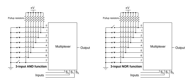
As we apply all possible high/low combinations to the three "select" input lines  $(S_2, S_1, \text{ and } S_0)$  of these multiplexers, those binary values select one input channel at a time (e.g. when  $S_2$  is low and  $S_1$  is low, and  $S_0$  is low, the mux selects the logic state applied to input terminal 0 to be "steered" to the output terminal.
