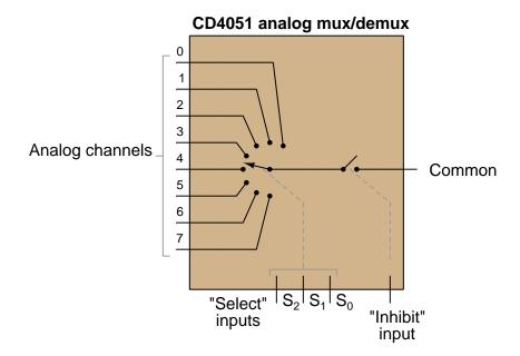
All digital inputs (the three select bits plus the inhibit) are active-high. Therefore, making the inhibit input pin high forces the internal MOSFET on the common terminal to turn off and places the device into an analog "high-impedance" mode where none of the eight analog channels connects to the common pin, while making the inhibit pin low connects the common pin to whichever analog channel is selected by the three select bits.
