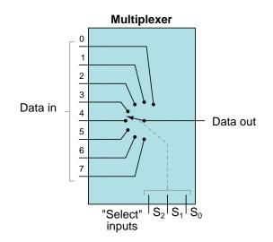
The three selector input lines accept a 3-bit binary number specifying which input channel's signal will be directed to the output (i.e. 000 selects input zero and 111 selects input seven).
