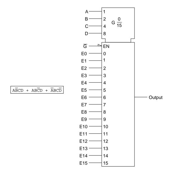
Show the wire connections necessary to make the multiplexer implement the specified Boolean expression.
