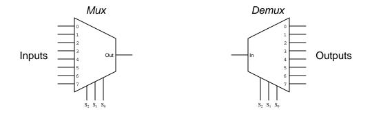
In the above illustrations we see 8-channel mux and demux functions, each with 3-bit selector words. Note how each of the selected I/O lines is numbered in decimal form according to the binary value of the selector word, but that it is also appropriate to label in binary as well. This next example shows binary labeling of selectable I/O lines for both mux and demux devices:
