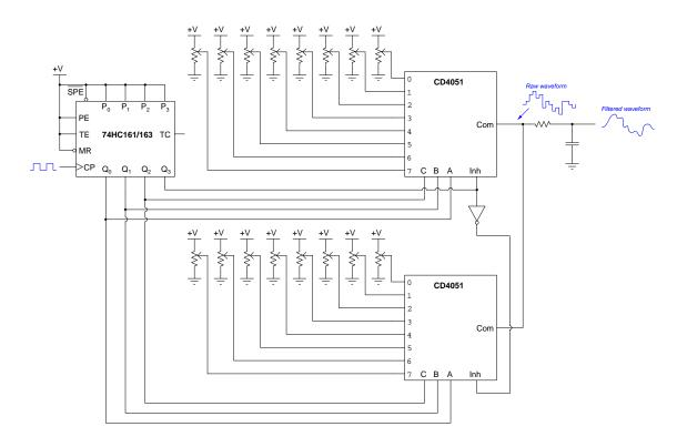
In this circuit, the counter's most-significant bit (MSB) output  $Q_3$  will be "low" during the first eight counts (0 through 7) and then "high" during the last eight counts (8 through 15), enabling the upper CD4051 mux for the first eight and the lower CD4051 mux for the latter eight count states. When each of these mux ICs are disabled, only the *other* mux will be able to send a potentiometer voltage value through to the RC filter.
