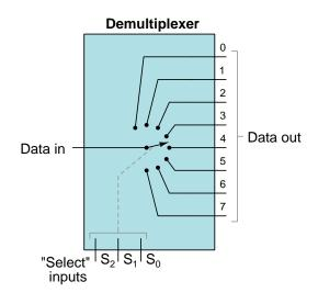
As with the mux, the demux's internal redirection logic is controlled by a binary word input, in this case a 3-bit binary value representing one of eight possible outputs.
