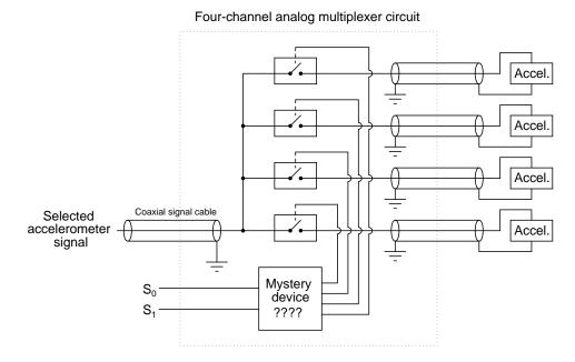
Identify the necessary "mystery device" shown in the schematic, which allows a binary input ( $S_0$  and  $S_1$  with four combinations of high/low states: 00, 01, 10, and 11) to activate just *one* bilateral switch at a time.
