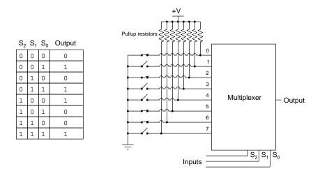
A simple thought experiment works well to explore how this circuit functions. Just imagine setting the three "select" input lines to various high (1) and low (0) states, one combination at a time, and see for yourself which input channel the mux selects for each combination. Remember that the three "select" input line states constitute bits of a three-bit binary number, the value of that number determining which input channel gets "steered" to the output:
