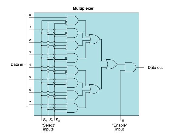
As with many combinational logic functions, multiplexers are often equipped with one or more *enable* or *strobe* inputs to override the output state regardless of channel or select line statuses. As you can see in the above diagram, the "enable" input allows data to pass through the multiplexer when active (high) but forces the output to a low state if inactive (low). Of course, you often find multiplexers with active-low enable inputs as well.
