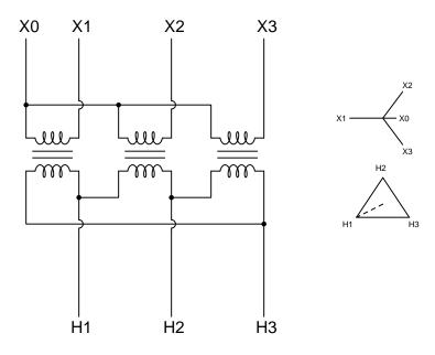
Which is the high-voltage side and which is the low-voltage side of this transformer? How can you tell?
