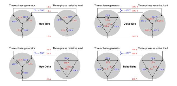
Note how phase and line currents are equal for all Wye networks because those quantities are in series with each other, and how phase and line voltages are equal for all Delta networks because those quantities are in parallel with each other. When currents combine at a node, or when voltages stack together, the result is a line quantity  $\sqrt{3}$  times greater than the phase quantity.
