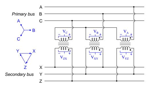
The resulting polyphase transformer bank converts the primary power (with "A-B-C" phase rotation) to secondary power with a "Z-Y-X" phase rotation<sup>1</sup>. The phase shift between primary voltage  $V_A$  (line A to ground) versus secondary voltage  $V_X$  (line X to ground) happens to be 90° with X lagging behind A.
