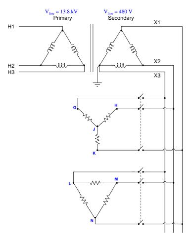
Determine the following phase-to-ground voltages in this system while both loads are energized:
