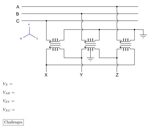
• Identify an alternative grounding method for the secondary windings than what is shown here.
