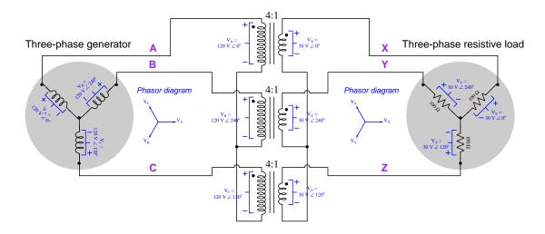
This means each of the 100-Ohm resistors in the "Wye" load receives 30 Volts AC, resulting in a current of 0.3 Amperes (both line and phase current, since those two quantities are equal in "Wye" networks). Each transformer secondary winding therefore carries the same 0.3 Amperes of current, which is stepped down to become a primary winding current of 75 milliAmperes AC. This becomes the phase and line current for the "Wye" source.
