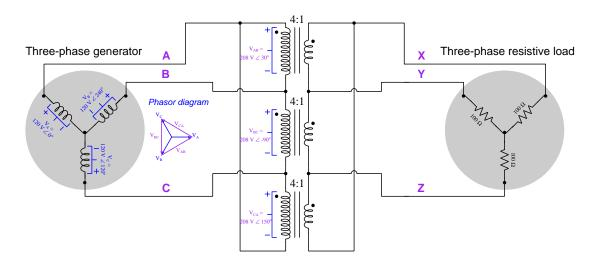
For example, on the upper-most transformer which has the "polarity" (dot) terminal connected to A and the "non-polarity" (non-dot) terminal connected to B, we sketch its phasor with tip touching A and tail touching B, and from that sketch we derive the proper angle for the voltage value written next to that winding (+ representing the phasor tip and - representing the phasor tail).
