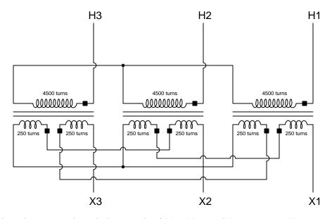
Calculate the magnitude and phase angle of  $V_{X1}$ ,  $V_{X2}$ , and  $V_{X3}$  assuming  $V_{H1}$  is 7.2 kV  $\angle 0^{\circ}$  and the phase rotation is H1-H2-H3.
