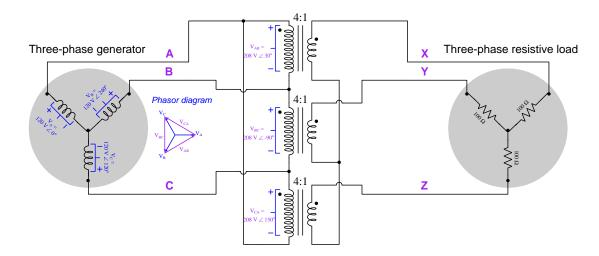
For example, on the upper-most transformer which has the "polarity" (dot) terminal connected to A and the "non-polarity" (non-dot) terminal connected to B, we sketch its phasor with tip touching A and tail touching B, and from that sketch we derive the proper angle for the voltage value written next to that winding (+ representing the phasor tip and - representing the phasor tail).
