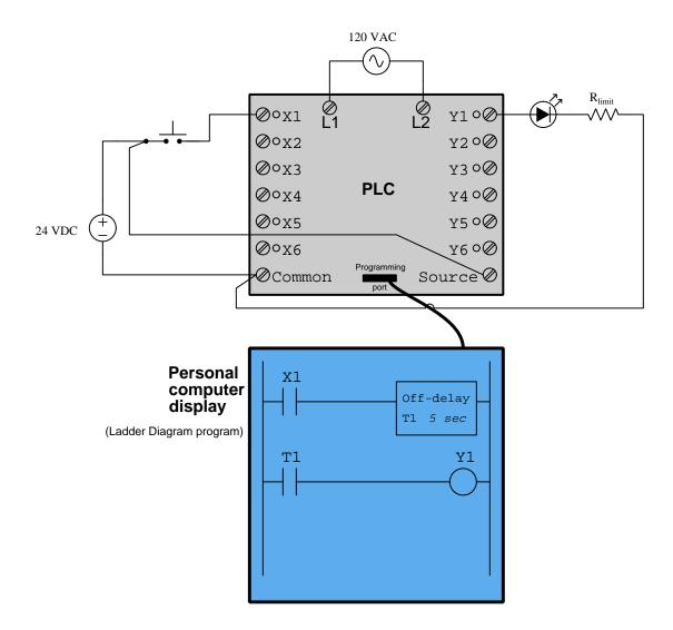
This program introduces a new label, T, associated with timer functions. Here, the virtual "contact" T1 is actuated by the timer function: immediately when X1 closes, and for an additional five second period of time following X1 returning to its resting (open) state.
