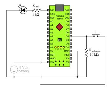
An optional 9 Volt battery provides electrical energy so that the Arduino may run independent of any other computer. When plugged into a programming computer's USB port, the Arduino draws power from that computer and requires no battery of its own.
