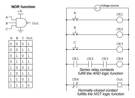
If any of the three inputs are low, the output goes high.
