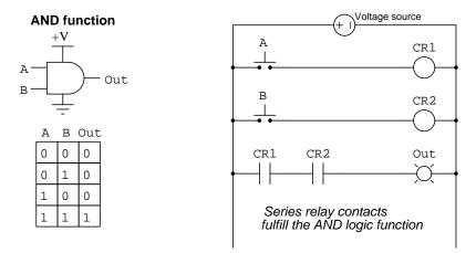
Both input A and input B must go to a "high" state (active) to make output "high" (active).
