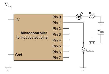
Next, we see one way to implement an off-delay timing function using a microcontroller:
