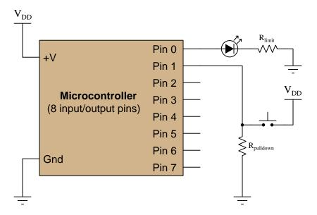
Next, we see one way to implement an on-delay timing function using a microcontroller:
