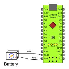
A USB port on the Arduino provides connection to a personal computer, where development software runs to allow the user to write code and download it into the microcontroller's memory. Once programmed and connected to a suitable source of electrical power, the microcontroller will then execute its program independent of any other computer.
