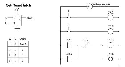
Input A acts to "set" the latch circuit and activate its output. Input B acts to do the opposite, "resetting" the latch and de-activating its output. When neither input A nor input B is activated, the latch circuit holds in its prior state – in other words, it *latches* to that prior state. In both of these circuit examples, input B has priority over input A, which means if both inputs are activated simultaneously, the circuit resets.
