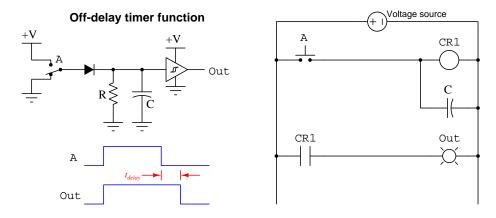
In both of these circuits, activation of the input (A) results in the capacitor immediately receiving a full "charge" of energy. In the semiconductor circuit this charge maintains a high state at the buffer gate's input terminal, forcing its output high as well. In the relay circuit this charge maintains voltage across relay coil CR1, actuating its normally-open contact and forcing it closed to illuminate the lamp.
