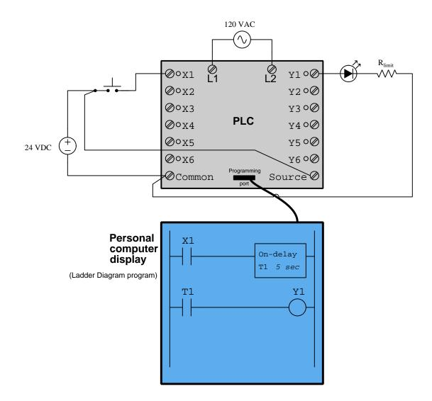
The T1 virtual "contact" is actuated by the timer function: five seconds after continuous closure of "contact" X1, returning to its resting (open) state immediately as the timing function is de-energized by the opening of "contact" X1.
