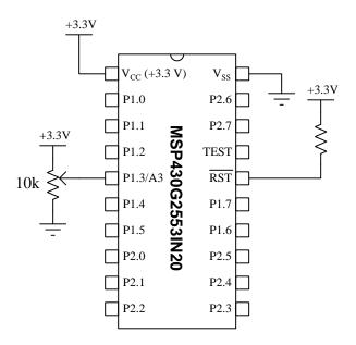
On the next page is a listing of the entire C-language code, tested and run on a Texas Instruments model MSP430G2553IN20 microcontroller using a LaunchPad model MSP-EXP430G2ET development board and version 10 of Code Composer Studio (CCS) in Debug mode.
