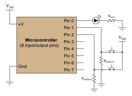
Next, we see how to implement the same logical latch function using a microcontroller:
