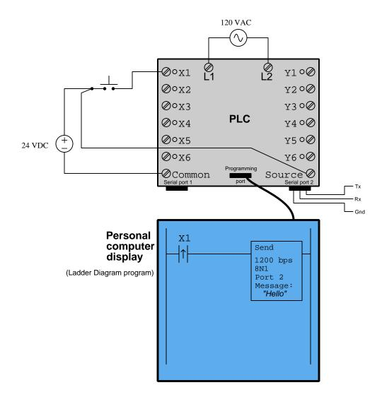
A "transition" or "edge" style of contact instruction is used for X1, so that the Send function is activated only *once* every time the pushbutton switch connected in input terminal X1 is pressed. If the Send function were continually activated, it is likely that the instruction would be re-executed before it had time to send the first message, which would result in a garbled message.
