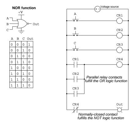
If any of the three inputs are high (active), the output goes low.
