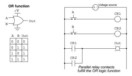
If either input A or input B is high (active), the output becomes high (active) as well.
