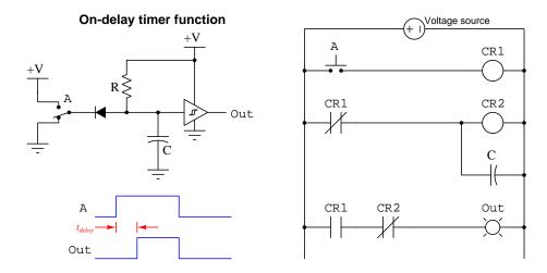
In both of these circuits, activation of the input (A) results in the capacitor's voltage either growing (gate circuit) or decaying (relay circuit) over time. When the capacitor voltage achieves a certain level, the output finally goes high in response to the input.
