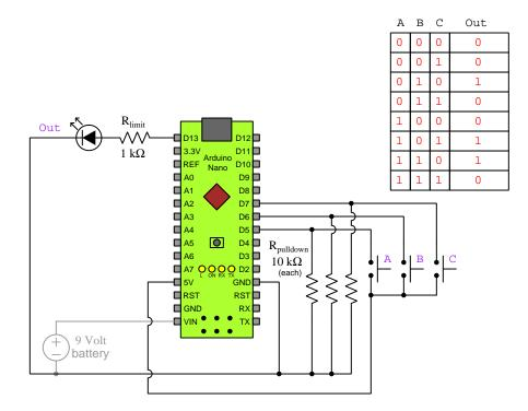
An optional 9 Volt battery provides electrical energy so that the Arduino may run independent of any other computer. When plugged into a programming computer's USB port, the Arduino draws power from that computer and requires no battery of its own.
