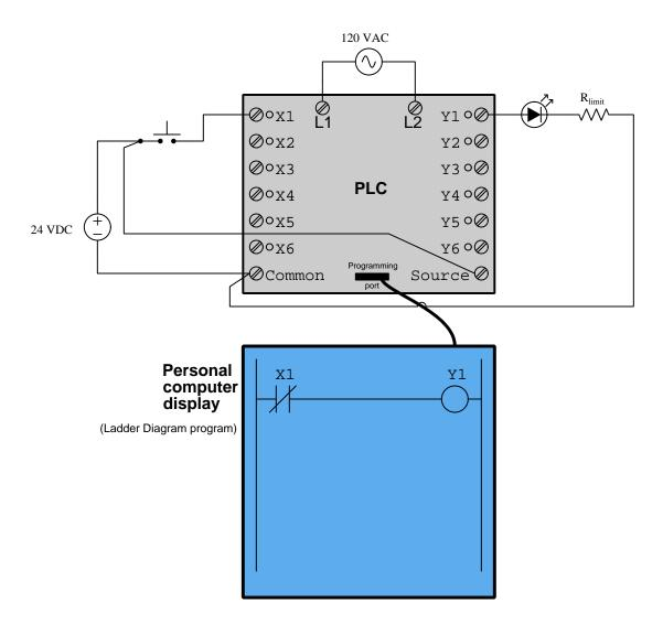
The virtual ladder-diagram "circuit" has just one "contact", and it is normally-closed which means is passes virtual "electricity" to output coil Y1 when in its resting state, which will be when input X1 is de-energized. If someone presses the pushbutton to energize input X1, the virtual contact X1 will be forced "open" which prevents virtual electricity from reaching coil Y1, thereby de-energizing the LED.
