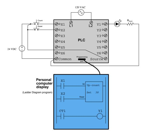
This PLC program energizes the LED if the count value meets or exceeds 38, just like the microcontroller program shown previously.
