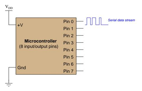
The blue-colored pulse waveform depicted here represents a sequence of "high" and "low" logic states represented as a voltage changing from full  $V_{DD}$  voltage ("high") to ground potential ("low") and back again. Viewed on an oscilloscope display, a serial data stream is a pulse waveform.
