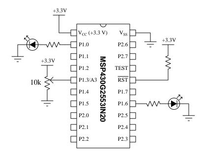
On the next page is a listing of the entire C-language code, tested and run on a Texas Instruments model MSP430G2553IN20 microcontroller using a LaunchPad model MSP-EXP430G2ET development board and version 10 of Code Composer Studio (CCS).
