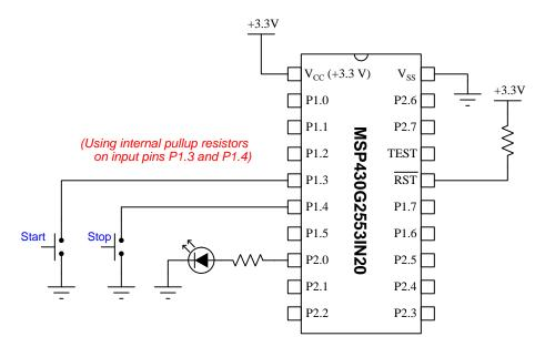
On the next page is a listing of the entire C-language code, tested and run on a Texas Instruments model MSP430G2553IN20 microcontroller using a LaunchPad model MSP-EXP430G2ET development board and version 10 of Code Composer Studio (CCS).
