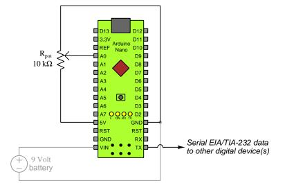
An optional 9 Volt battery provides electrical energy so that the Arduino may run independent of any other computer. When plugged into a programming computer's USB port, the Arduino draws power from that computer and requires no battery of its own.
