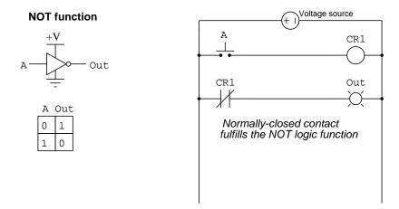
In these circuits the output state is exactly opposite of the input, the NOT function *complementing* the input's state.
