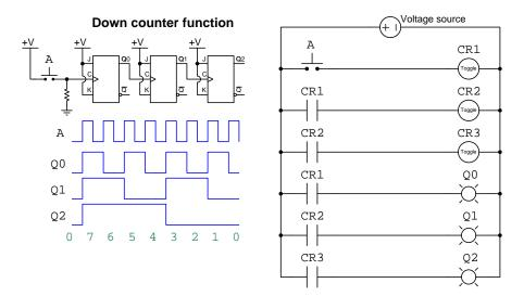
Also, there are *up-down counters* with two different inputs, either one to increment and another to decrement the accumulated count value, or one to trigger the count and another to command the direction of that count.
