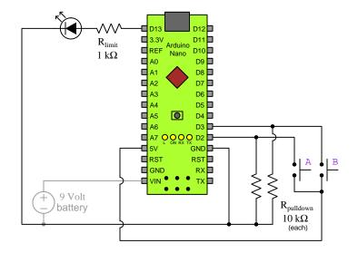
**Functional behavior** – microcontroller counts the number of times pushbutton **A** is pressed and activates the LED if that number is equal to or greater than five.
