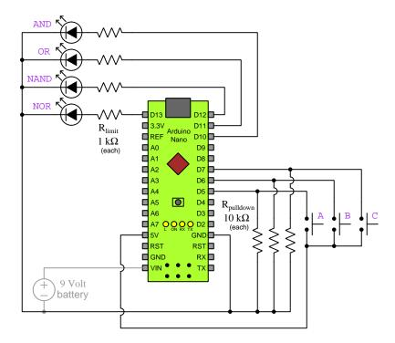
An optional 9 Volt battery provides electrical energy so that the Arduino may run independent of any other computer. When plugged into a programming computer's USB port, the Arduino draws power from that computer and requires no battery of its own.
