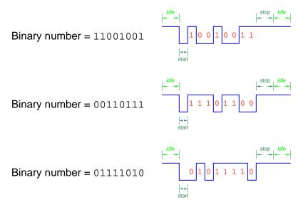
Next we will examine three more examples of UART signals using the same parameters as before (positive logic levels, 8 data bits, and 2 stop bits), but this time including a *parity bit* set for *odd parity*:
