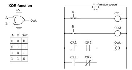
If the logical states of input A and input B differ, the output goes high; otherwise the output will be low.
