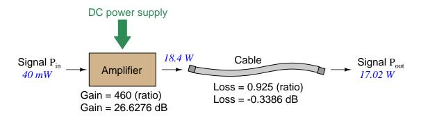
The overall gain of this amplifier and cable system expressed as a ratio is equal to the *product* of the individual component gain/loss ratios. That is, the gain ratio of the amplifier *multiplied* by the loss ratio of the cable yields the overall power ratio for the system:
