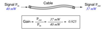
$$10\log\left(\frac{P_{out}}{P_{in}}\right) = 10\log\left(\frac{37 \text{ mW}}{40 \text{ mW}}\right) = -0.3386 \text{ dB}$$
