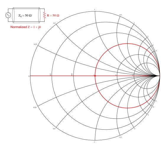
This is the point marked by the intersection of the "1" resistance circle and the "0" reactance circle (i.e. a "circle" with an infinite radius which is really a straight line overlapping the horizontal axis).
