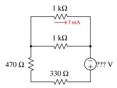
Here, the source's voltage value is unknown, but current through one of the resistors is provided.
