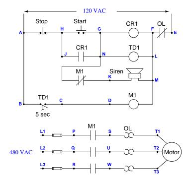
Each student has their own copy of the diagram, as does the instructor. The instructor has furthermore identified a realistic fault within this system, and has full knowledge of that fault's effects. In other words, the instructor is able to immediately tell a student how much voltage will be read between any two test points, what the effect of jumpering a pair of test points will be, what will happen when a pushbutton is pressed, etc.
