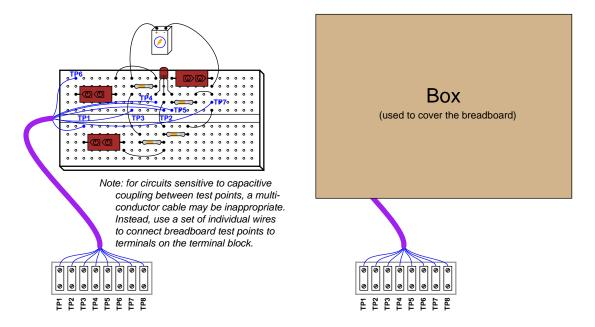
If students cannot visually detect a fault, they must rely on voltage measurements taken from terminals on the block. This is quite challenging, as not even the shapes of the components may be seen with the box in place. The only guide students have for relating terminal block test points to points in the circuit is the schematic diagram, which is good practice because it forces students to interpret and follow the schematic diagram.
