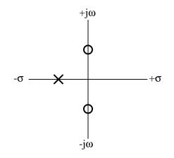
Whether an RLC network is over-damped, under-damped, or critically damped depends on the mathematical sign of the *discriminant*, that portion of the quadratic equation contained within the radicand:
