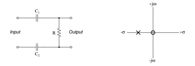
Transfer function =  $\frac{sRC_1C_2}{sRC_1C_2 + C_1 + C_2}$
