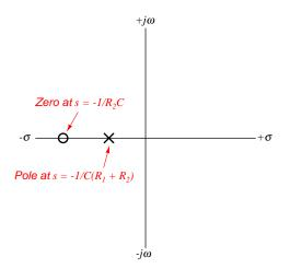
If we happen to know the actual component values for C,  $R_1$ , and  $R_2$ , we may compute complex frequency values for the network's zero and pole. Supposing C is 10 microFarads,  $R_1$  is 1 kiloOhm, and  $R_2$  is 2.2 kiloOhms, the zero and pole frequencies for this particular network will be as follows<sup>1</sup>:
