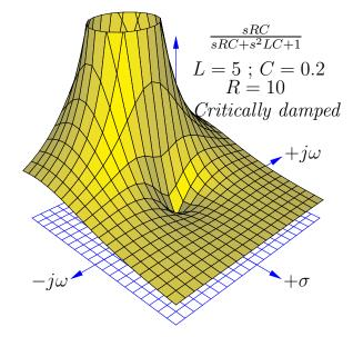
First, the critically-damped example, with a resistor value of 10 Ohms:
