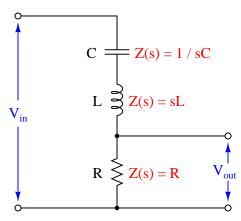
As usual, the transfer function for this circuit is the ratio between the output component's impedance (R) and the total series impedance, functioning as a voltage divider:
