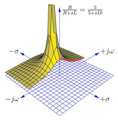
Only one-half of the pole-zero surface has been plotted here, in order to better reveal the crosssection along the  $j\omega$  axis. The bold, red curve traces the edge of the transfer function surface as it begins at zero frequency (DC) to increasingly positive values of  $j\omega$ . The red trace is therefore the Bode plot for this low-pass filter, starting at a maximum value of 1 ( $V_{out} = V_{in}$  for a DC input signal) and approaching zero as frequency increases.
