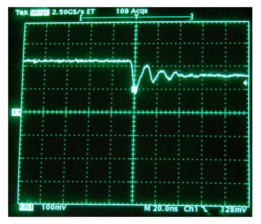
Determine the complex frequency of the "ringing" observed in this AC voltage signal:
