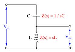
Writing the transfer function for this tank circuit is (once again) a matter of expressing the ratio between the output component's impedance versus the total circuit impedance:
