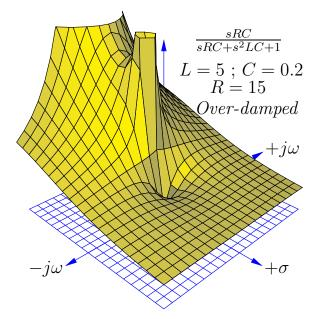
We clearly see *two* poles<sup>13</sup> centered along the  $\sigma$  axis in this plot, representing the two real roots of the transfer function's denominator. Again, we will use the quadratic formula to solve for these two values of s:
