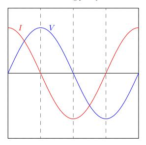
Therefore, when we apply a sinusoidal voltage across a pure capacitance, the current waveform is also a sinusoid but phase-shifted by 90 degrees leading. In other words, *current leads voltage by 90 degrees for a pure capacitance*.
