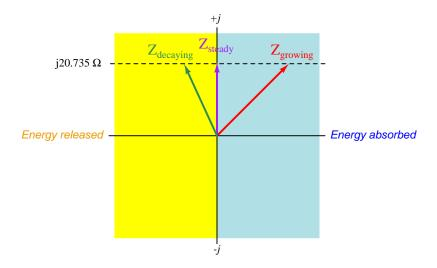
In all three cases the imaginary portion of the impedance is the same (j20.735 Ohms), but the growth or decay of the signal over time contributes a net absorption or net release, respectively, of energy by the inductor over multiple cycles.
