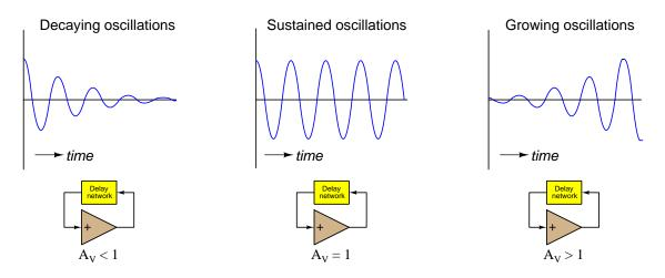
Sketch locations of poles for each of these oscillator loop-gain conditions, qualitatively placing "X" marker(s) for those locations on the s plane:
