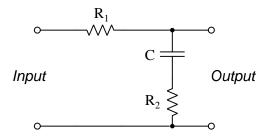
This network's transfer function may be written using the voltage divider equation, placing the series impedance of C and  $R_2$  over the total network impedance as seen from the input terminals. First, writing an s-domain impedance equation for C and  $R_2$ :
