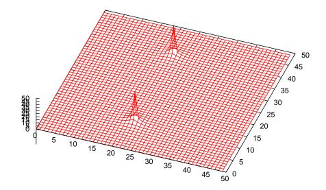
This particular simulation uses increments of 0.04 per second (incr in the C++ code), which is the value of each division (space between lines) on the two horizontal axes. The two poles of this filter network are clearly evident in the three-dimensional plot, but the height of these peaks is quite irrelevant to our purposes. We just want to know how many poles there are, and where those poles are located on the *s* plane.
