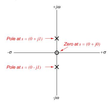
The placement of these poles on the imaginary axis means their real values are zero, which in turn means the oscillations neither grow nor decay over time. This, of course, is possible only for an LC network with no parasitic losses (e.g. resistance) whatsoever. If we were to include dissipative elements into the network we would see a decay rate as well, shifting the poles to the left so as to have negative real  $(-\sigma)$  values.
