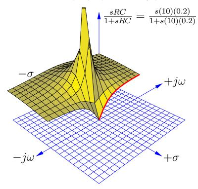
Once again the bold, red curve traces the edge of the transfer function surface as it begins at zero frequency (DC) to increasingly positive values of  $j\omega$ . The red trace is therefore the Bode plot for this high-pass filter, starting at a minimum value of 0 ( $V_{out} = 0$  for a DC input signal) and approaching unity (1) as frequency increases. Naturally, this is the type of response we would expect to see exhibited by a high-pass filter circuit.
