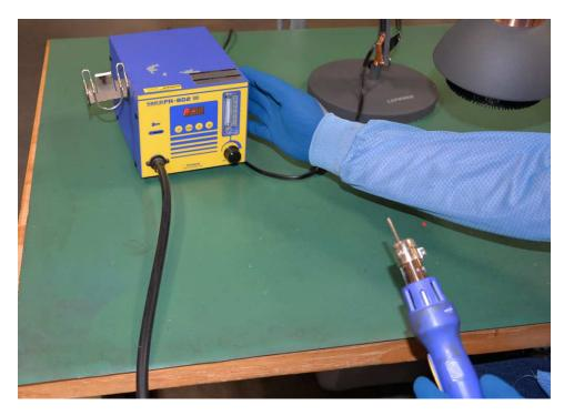
The bench-top portion of this hot air station contains the air blower, air flow monitor and control valve, and power electronics to drive the heating element inside the pencil portion. A cord containing an air tube and wiring connects the pencil to the bench-top portion.
