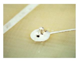
Another potential source of blowholes is excessive flux applied to a joint prior to the application of molten solder. Since flux vaporizes with the application of soldering heat, this vapor needs a route to escape, and if there is too much flux applied prior to soldering (either in liquid or paste form), some of that flux vapor will escape as bubbles through the molten solder, potentially leaving voids or holes in its wake.
