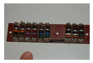
Note how the shape of each of the resistors' leads may be seen beneath the layer of solder, showing each wire partially wrapped around a notched metal tab for mechanical integrity. The metal tabs are anchored to a fiberglass board (similar to printed circuit board material) which is electrically non-conductive.
