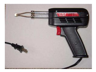
Soldering guns generally have much greater power ratings than soldering irons, in most cases exceeding 100 Watts. They are most useful when soldering large-gauge copper wires. Unlike soldering irons which typically remain powered, soldering guns are trigger-activated which means they de-energize whenever you let go of the trigger with your finger. This is good, as the guns are usually rated for intermittent use only.
