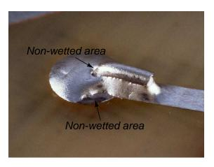
Below we see another photograph  $^{13}$  of a solder joint having non-wetted areas, as well as visible stress lines on the surface of the solder:
