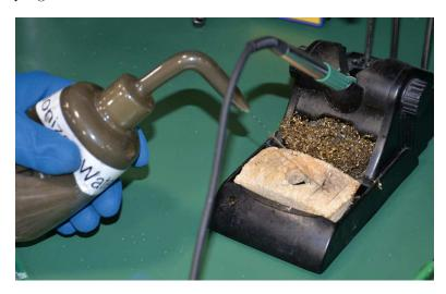
A well-maintained soldering iron tip should have a shiny metallic surface. Oxidation usually appears dark in color, and serves as a good visual indicator that cleaning is necessary.
