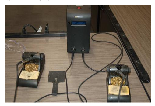
This particular soldering station is made by Metcal, and features two soldering irons in their own holders. It is a professional-grade unit with a high power output of approximately 75 Watts which means the iron tip(s) will reach full temperature within just a few seconds of applied power, and also that they will be able to maintain proper soldering temperature even when making thermal contact with large areas of copper on a circuit board that behave like a natural heat sink.
