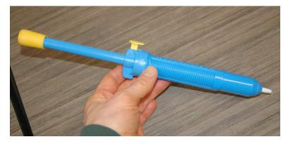
These tools work well to clear out through-hole pads in printed circuit boards, by applying suction to the hole on one side of the PCB and soldering-iron heat to the other side.
