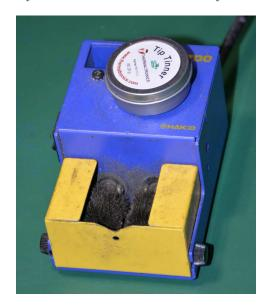
Generally speaking, good tip-maintenance habits such as regularly tinning the tip with solder to guard against oxidation should make tip tinner and brush tools unnecessary. However, for low-quality and/or mis-treated soldering iron tips they may be useful.
