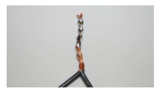
It should be clear from this photograph how the solder has filled the spaces between the two twisted wire ends, thereby greatly increasing the amount of surface area connecting the two wires together. The metallic bonding between the copper wire and the solder alloy also greatly strengthens the splice and prevents corrosion by positively displacing all air and moisture from reaching the copper wire surfaces.
