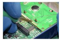
Soldering the terminals of a surface-mount component onto copper pads on a printed circuit board is much the same, in that applying the soldering iron's heat to the copper pad and letting that heat flow into the component lead is generally a good strategy. Here we see one tab of a lithium "button" style battery holder being soldered onto a PCB:
