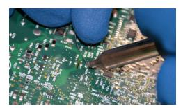
Here you can see the solder wire plainly being added while heating the work to be de-soldered. That added solder simply gets sucked up into the desoldering tool along with the rest of the solder that came from the work. The degree to which this tool is able to draw solder away from a PCB and out of its through-holes is impressive, as shown in the next photograph after a four-terminal through-hole component has been removed from a PCB:
