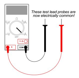
Touching the meter's test leads to two points in a circuit will now "jumper" those two points together, any current flowing through the shunt resistance of the multimeter. If desired, the meter may be turned on to monitor how much current goes through the "jumper" if this is diagnostically relevant.
