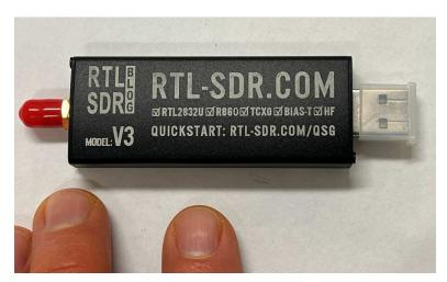
The single most important piece of advice I have for using the RTL-SDR module is to utilize a USB extension cable when connecting it to your computer's USB port, as the device itself is rather long and heavy and will place mechanical strain on that connector if directly plugged in.
