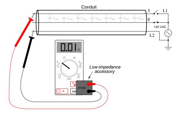
With the voltmeter's input impedance artificially decreased by the application of this accessory, the capacitive coupling is insufficient to produce any substantial voltage dropped across the voltmeter's input terminals, thus eliminating. The technician may now proceed to test for the presence of AC control signal (or power) voltages with confidence.
