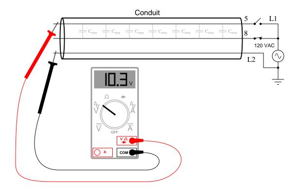
With the power switch feeding wire 5 in the open state, there should be no AC voltage measured between wire 5 and neutral (L2), yet the voltmeter registers slightly over 10 volts AC. This "phantom voltage" is due to capacitive coupling between wire 5 and wire 8 (still energized) throughout the length of their mutual paths within the conduit.
