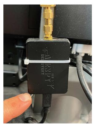
Airspy provides a simple-to-use server for sending the receiver's I-Q data stream over a TCP/IP network, which makes it particularly useful for distributed applications with a remote-mounted receiver.
