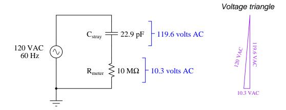
An analog voltmeter would never have registered 10.3 volts under the same conditions, due to its substantially lower input impedance. Thus, "phantom voltage" readings are a product of modern test equipment more than anything else.
