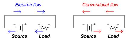
Whichever notation you choose to follow in your analysis of circuits, the understanding should be the same: the reason voltage polarities across the resistor and battery differ despite the same direction of current through both is the flow of power. The battery acts as a *source*, while the resistor acts as a *load*.
