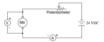
When operating the motor at a voltage of 16 volts and a current of 2 amps, though, smoke begins to pour out of the potentiometer, indicating that its power rating is being exceeded.
