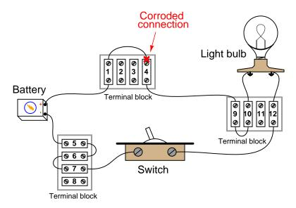
Taking voltage measurements with a voltmeter, how do you think this corrosion problem will reveal itself with the switch on the ON position? In other words, which voltage measurement in this circuit (i.e. between which pair or pairs of terminal block points) will be unusual as a result of the bad connection at point #4, and approximately how much voltage should that measurement be?
