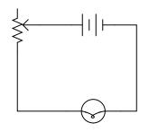
For a 9 volt battery, there will be  $1.44\times10^{-18}$  joules of energy imparted to each electron moving through it.
