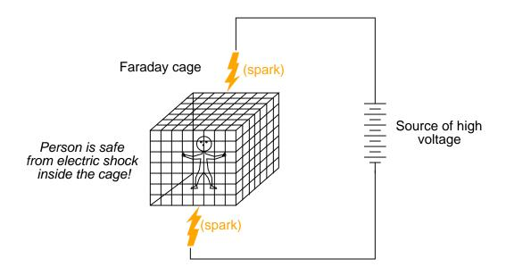
Explain how the principle of electrically common points protects the person inside the Faraday cage from being shocked by the outside source of high voltage. Discuss how this principle might apply to metal-frame automobiles and aircraft.
