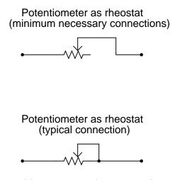
Explain what advantage is gained by connecting the wiper to the unused terminal. Why is the lower potentiometer connection scheme more commonly used than the upper? <u>file 00343</u>
