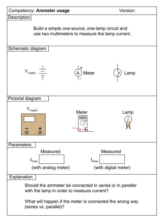
**IMPORTANT NOTE:** do not actually try to connect the ammeter improperly in the circuit, as the meter may be damaged in the process! <u>file 01714</u>
