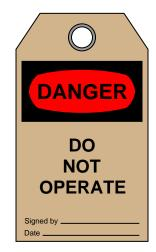
What is the purpose of attaching such a tag to an electrical disconnect device in addition to locking it in the open position? Why is a lock, by itself, not sufficient from a safety perspective? <u>file 00573</u>
