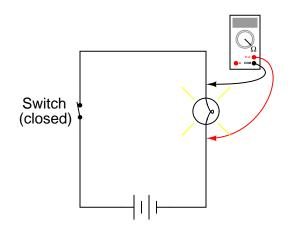
Suppose we needed to determine the resistance of the light bulb in this circuit, while energized:
