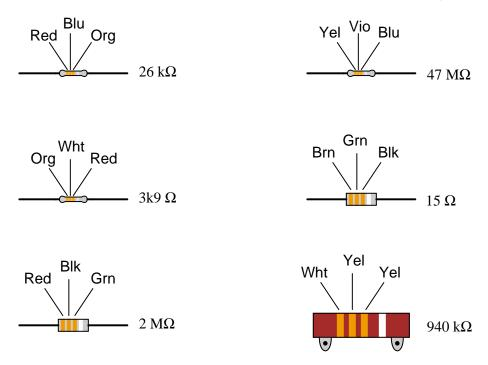
What patterns do you notice between the color codes (given as three-letter abbreviations, so as to avoid interpretational errors resulting from variations in print quality), the resistance values, and the physical sizes of the resistors? <u>file 00216</u>
