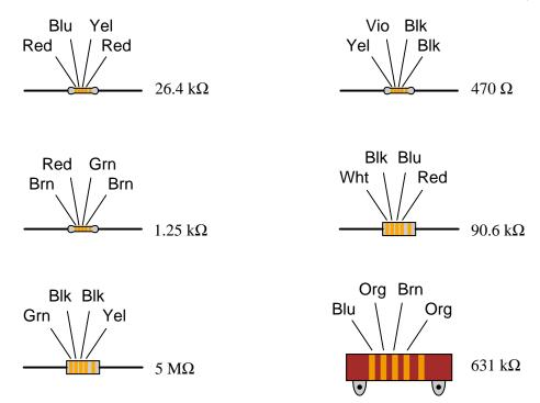
What patterns do you notice between the color codes (given as three-letter abbreviations, so as to avoid interpretational errors resulting from variations in print quality) and the resistance values of each resistor? Why do precision resistors use a "5-band" color code instead of a "4-band" color code? file 00265
