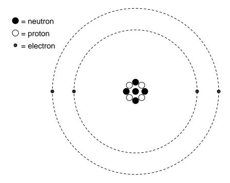
Although electrons are present in all atoms, and therefore in all normal substances, the outer electrons in conductive substances are freer to leave the parent atoms than the electrons of insulating substances. Such "free" electrons wander throughout the bulk of the substance randomly. If directed by a force to drift in a consistent direction, this motion of free electrons becomes what we call *electricity*.
