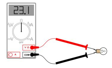
Also, identify the reading you would expect the ohmmeter to indicate if the light bulb were burnt out (failed "open"). file 00101
