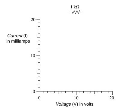
Plot this graph, following Ohm's Law. Then, plot another graph representing the voltage/current relationship of a 2 k $\Omega$  resistor.
