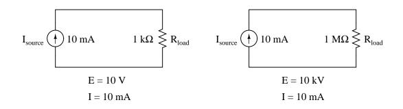
Follow-up question: identify the polarity of the voltage drops across the resistors in the circuits shown above.
