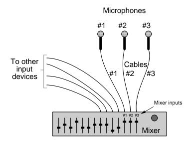
The purpose of the mixer is to function as a multi-channel audio signal amplifier, to control the volume of each sound channel so that a good "mix" is obtained for recording. The studio engineer will use the individual controls on the mixer to "blend" the inputs for the best recording tone and quality.
