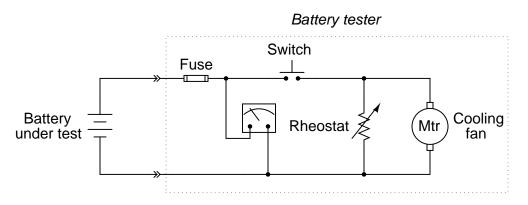
Other clues to the problem include the fact that rheostat setting seems to make no difference in the voltmeter's indication, and also that the cooling fan motor does not come on when the switch is pressed.
