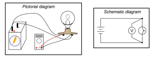
In order to practically function, an voltmeter must have some finite amount of internal resistance. It is usually a very large amount, but less than infinite. It should be apparent to you that the presence of this resistance will have some effect on the circuit voltage, when compared to the amount of voltage in the circuit without any meter connected, due to the fact that real voltage sources tend to "sag" when subjected to additional loads:
