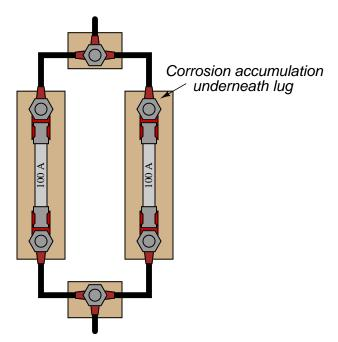
Explain how a small accumulation of corrosion led to this condition of fuses blowing when there was no overcurrent condition (load current less than 200 amps), and also why connecting fuses in parallel like this is generally not a good idea.
