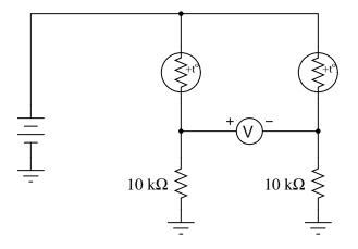
The "+t°" label in each one shows that they both have positive  $\alpha$  coefficients.
