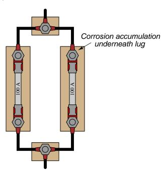
Explain how a small accumulation of corrosion led to this condition of fuses blowing when there was no overcurrent condition (load current less than 200 amps), and also why connecting fuses in parallel like this is generally not a good idea.
