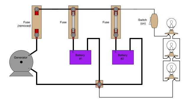
The two batteries are rated such that they are supposed to provide at least 10 hours of back-up power in the event of a generator "outage" such as this. Unfortunately, the light bulbs begin to dim much sooner than expected. Something is wrong in the system, and you are asked to figure out what.
