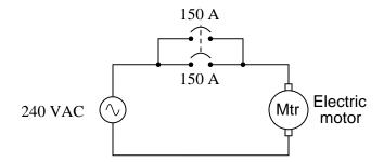
An electrician measures motor current using a clamp-on ammeter, and discovers the motor's current is no more than 228 amperes at full mechanical load. Describe what might possibly be wrong that is causing both circuit breakers to trip.
