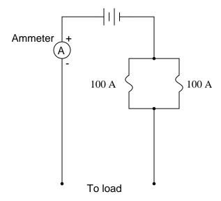
However, after a few years of operation, the system begins blowing fuses even when the ammeter registers less than 200 amps of load current. Upon investigation, it is found that one of the fuse holders had developed corrosion on a terminal lug where one of the wire connects:
