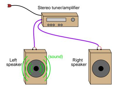
Identify three possible faults that could cause this problem to occur, and identify what components of the stereo system are known to be okay (be sure to count each cable as a separate component of the system!).
