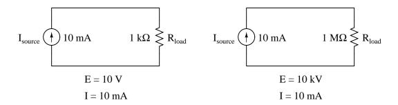
Follow-up question: identify the polarity of the voltage drops across the resistors in the circuits shown above.
