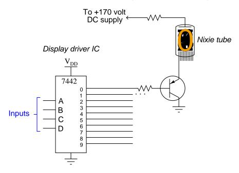
Unfortunately, that one digit begins to glow the moment the high-voltage DC supply is turned on, even before the 7442 chip receives power! And after that, the 7442 gets warm to the touch, which is not good.
