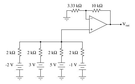
Calculate the necessary resistor value  $(R_1)$  in this circuit to give it a voltage gain of 10.5:
