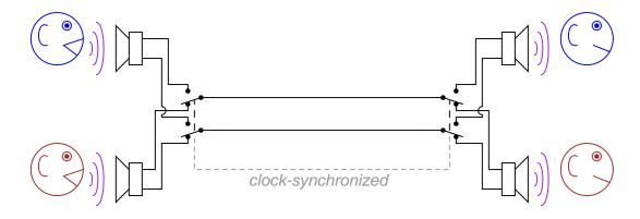
What would the conversation sound like to either of the listeners if the switch frequency was 1 Hz? What if it was 10 Hz? What if it was 40 kHz?  $\frac{\text{file }01343}{\text{file }01343}$
