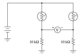
The "+ $t^{o}$ " label in each one shows that they both have positive  $\alpha$  coefficients.
