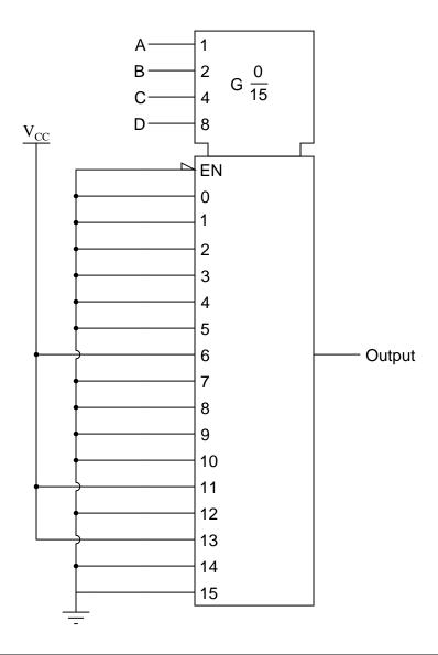
In the first scenario with the enable lines grounded, output #11 will be low, with all other outputs high. In the second scenario with a square wave signal input to the enable lines, output #11 will pulse while all other outputs remain in the high state.
