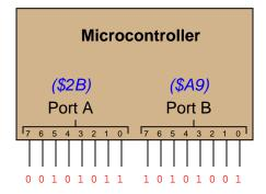
Suppose we wished to use the first seven bits of each port (pins 0 through 6) to drive two 7-segment, common-cathode displays, rather than use BCD-to-7-segment decoder ICs:
