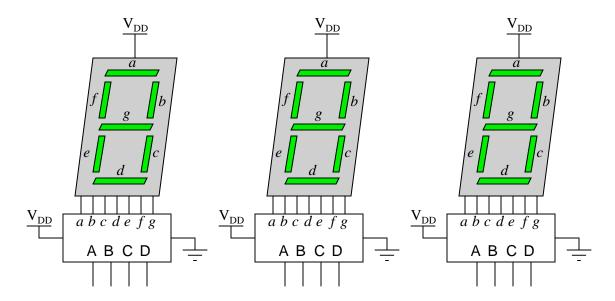
If we are driving the decoder ICs with a microprocessor or microcontroller, this direct technique unfortunately uses a lot of I/O pins. In this particular case, with three 7-segment displays, we would need to use twelve output pins on the microcontroller for the three BCD numbers:
