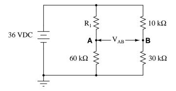
How much resistance must  $R_1$  possess in order to drop that amount of voltage? file 00543
