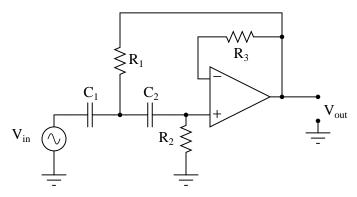
Determine which of these Sallen-Key filters is low pass, and which is high pass. Explain your answers.  $\underline{\text{file }00765}$
