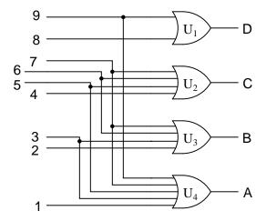
Predict how the operation of this "flash" analog-to-digital converter (ADC) circuit will be affected as a result of the following faults. Consider each fault independently (i.e. one at a time, no multiple faults):
