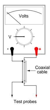
When measuring high-frequency AC voltages, however, the parasitic capacitance and inductance of the coaxial cable may present problems. We may represent these distributed characteristics of the cable as "lumped" parameters: a single capacitor and a single inductor modeling the cable's behavior:
