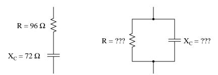
Note that I have already provided a value for the capacitor's reactance  $(X_C)$ , which of course will be valid only for a particular frequency. Determine what values of resistance (R) and reactance  $(X_C)$  in the parallel network will yield the exact same total impedance  $(Z_T)$  at the same signal frequency. file 01540
