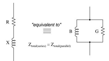
We know that resistance (R), reactance (X), and impedance (Z), as scalar quantities, relate to one another trigonometrically in a series circuit. We also know that conductance (G), susceptance (B), and admittance (Y), as scalar quantities, relate to one another trigonometrically in a parallel circuit:
