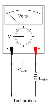
Typical parasitic values for a 10-foot cable would be 260 pF of capacitance and 650  $\mu$ H of inductance. The voltmeter itself, of course, is not without its own inherent impedances, either. For the sake of this example, let's consider the meter's "input impedance" to be a simple resistance of 1 M\Omega.
