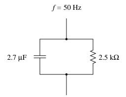
Also, express the total impedance of either circuit (since they are electrically equivalent to one another, they should have the same total impedance) in *complex form*. That is, express  $\mathbf{Z}$  as a quantity with both a magnitude and an angle.
