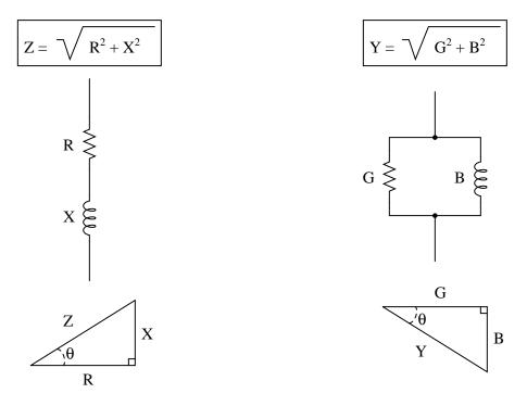
If these two circuits are truly equivalent to one another, having the same total impedance, then their representative triangles should be geometrically similar (identical angles, same proportions of side lengths). With equal proportions,  $\frac{R}{Z}$  in the series circuit triangle should be the same ratio as  $\frac{G}{Y}$  in the parallel circuit triangle, that is  $\frac{R}{Z} = \frac{G}{Y}$ .
