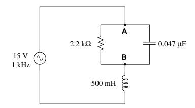
Hint: convert the parallel RC sub-network into a series equivalent first.  $\underline{\mathrm{file}~02115}$
