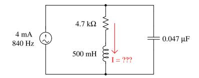
Hint: convert the series LR sub-network into a parallel equivalent first.  $\underline{\mathrm{file}~02116}$
