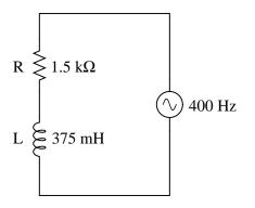
Also, express the total impedance of either circuit (since they are electrically equivalent to one another, they should have the same total impedance) in *complex form*. That is, express  $\mathbf{Z}$  as a quantity with both a magnitude and an angle.
