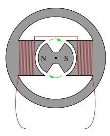
Hint: how many cycles of AC are produced for every revolution of the rotor? file 00819
