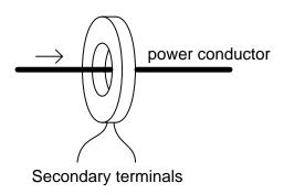
The purpose of a current transformer is to create a secondary current that is a precise fraction of the primary current, for easier measurement of current in the power conductor.
