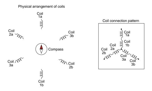
Hint: imagine the electromagnets were light bulbs instead, and the frequency of the AC power was slow enough to see each light bulb cycle in brightness, from fully dark to fully bright and back again. What would the pattern of lights appear to do?
