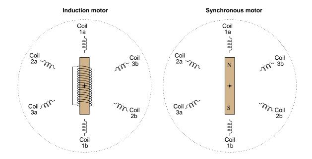
Synchronous AC motors use a permanent magnet rotor, while *induction* motors use an electromagnet rotor. Explain what practical difference this makes in each motor's operation, and also explain the meaning of the motors' names. Why is one called "synchronous" and the other called "induction"? file 00740
