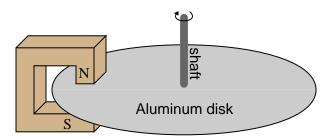
The disk itself need not be made of a ferromagnetic material in order for the magnet to create a "drag" force. It simply needs to be a good conductor of electricity.
