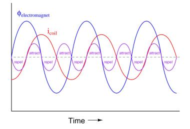
Note the equal-amplitude attraction and repulsion peaks shown on the graph.
