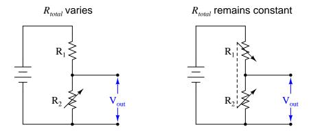
Knowing that the voltage output by a voltage divider is described by the following formula, determine which voltage divider circuit yields the greatest change in output voltage for a given change in  $R_2$ 's resistance.
