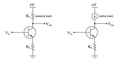
Usually, this "active load" takes the form of a current mirror circuit, behaving as a current regulator rather than as a true current source.
