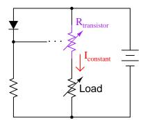
In other words, as  $R_{load}$  increases, what does  $R_{transistor}$  do – increase resistance, decrease resistance, or remain the same resistance it was before? How does the changing value of  $R_{transistor}$  affect total circuit resistance?
