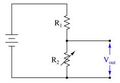
Suppose we were to compare the performance of two voltage divider circuits side-by-side. The circuit on the left has one variable resistor  $(R_2)$ , while the circuit on the right has two variable resistors  $(R_1)$  and  $(R_2)$ . The right-hand circuit's resistors are ganged together in such a way that as one resistance increases, the other will decrease by the same amount, keeping the circuit's total resistance constant:
