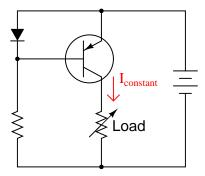
If we were to crudely model the transistor's behavior as an automatically-varied rheostat – constantly adjusting resistance as necessary to keep load current constant – how would you describe this rheostat's response to changes in load resistance?
