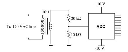
Unfortunately, this ADC is not able to fully sample the AC waveform when tested. It "overflows" and "underflows" at the waveform's peaks, as though the input waveform is too large (outside of the +5/-5 volt ADC chip range). The technician re-checks his calculations, but still thinks the voltage division ratio provided by the potential transformer and resistor network should be sufficient for this task.
