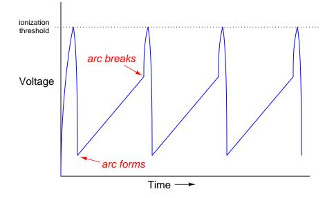
The most important point of this question, though, is to relate these principles to the topic of "arc blast". How does the dramatic decrease in air resistance (after ionization) relate to the magnitude of arc current? How does the motion of the arc in a Jacob's Ladder relate to the high temperatures of an arc? What about the difference in gaps between the bottom of the rods versus the top – how does this relate to the physical size of arcs in an electrical power system fault?
