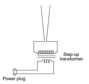
When powered, an arc develops at the point where the two rods are closest, then travels up the length of the rods, becoming wider and wider, until it "breaks" off the top of the rods. Once the arc is extinguished, a new arc forms at the bottom of the rods again.
