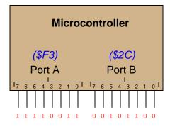
Suppose we wished to use the upper four bits of port A (pins 7, 6, 5, and 4) to drive the coils of a stepper motor in this eight-step sequence:
