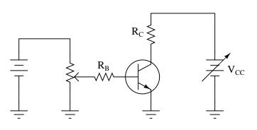
Procedure: measure the voltage dropped across  $R_C$  while varying  $V_{CC}$ , for several different values of  $I_B$  (inferred by measuring voltage drop across  $R_B$ ).
