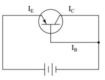
Which current is the smallest and which is the largest? Are there any two currents that are closer in magnitude than with the third? If so, which currents are they?
