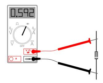
When using a multimeter with this feature to identify the terminals of a bipolar junction transistor, the forward voltage drop indication is necessary to distinguish the collector terminal from the emitter terminal. Explain how this distinction is made on the basis of the forward voltage measurement, and also explain why this is.
