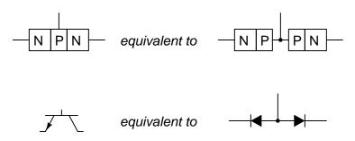
Acting on this idea, the student proceeds to connect two 1N4001 rectifying diodes back-to-back and try to use it as a transistor. This idea does not work: although the diode pair reads the same patterns of continuity as a transistor would, it does not amplify. Explain why.
