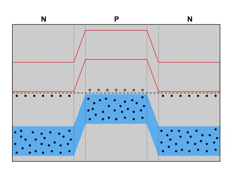
"Injection" current consists of those majority charge carriers (either electrons or holes, depending on the transistor type) that are "injected" from the emitter region into the base region of a transistor. "Diffusion" current is the current through the base terminal of the transistor resulting from recombination of electrons and holes in the emitter-base junction. Most of the injection current, however, becomes "collection" current and goes through the collector terminal of the transistor.
