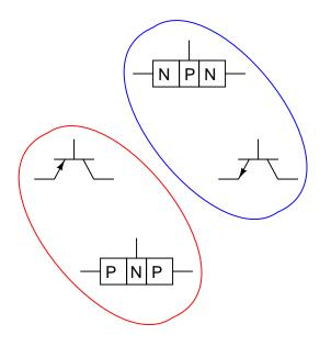
Follow-up question: identify the terminals on each transistor schematic symbol (base, emitter, and collector).
