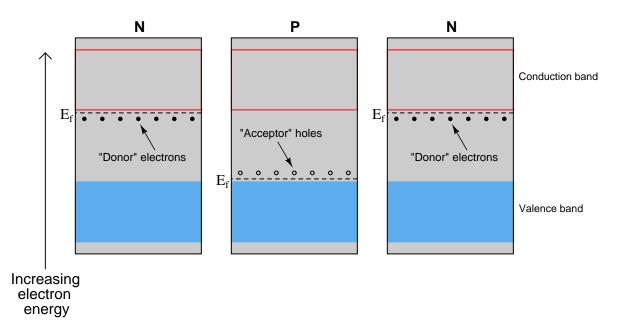
The presence of dopants in the semiconducting materials creates differences in the Fermi energy level  $(E_f)$  within each piece.
