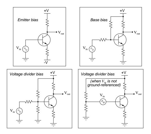
Each one has the same basic purpose, but works in a different way to accomplish it. Describe the purpose of any biasing network in an AC signal amplifier, and comment on the different means of accomplishing this purpose employed by each of the three circuits.
