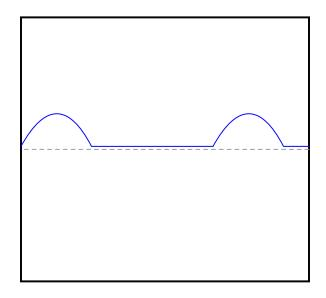
Definitely not Class-A operation! Suspecting a problem with the input waveform, the student disconnects the oscilloscope probe from the amplifier output and moves it over to the amplifier input terminal. There, the following waveform is seen:
