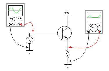
It should be apparent that only portions of the input are being reproduced at the output of this circuit. The rest of the waveform seems to be "missing," being replaced by a flat line. Explain why this transistor circuit is not able to amplify the *entire* waveform. <u>file 02222</u>
