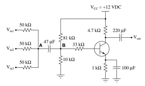
Suppose we measured a 9 kHz sinusoidal voltage of 0.5 volts (peak) at point "A" in the diagram, using an oscilloscope. Determine the voltage at point "B" in the circuit, after this AC signal voltage "passes through" the voltage divider biasing network.
