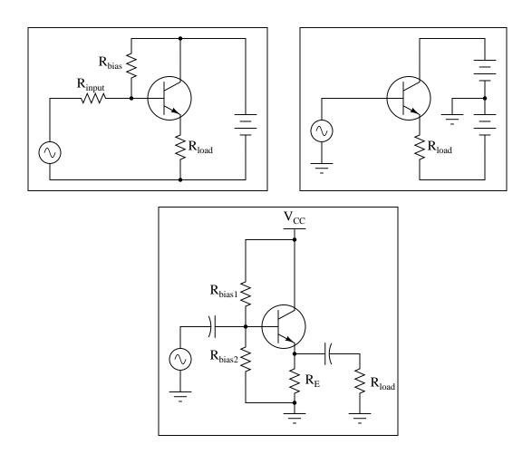
Each one has the same basic purpose, but works in a different way to accomplish it. Describe the purpose of any biasing network in an AC signal amplifier, and comment on the different means of accomplishing this purpose employed by each of the three circuits.
