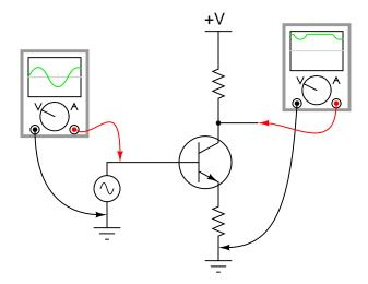
It should be apparent that only portions of the input are being amplified in this circuit. The rest of the waveform seems to be "missing" in the output, being replaced by a flat line. Explain why this transistor circuit is not able to amplify the entire waveform.
