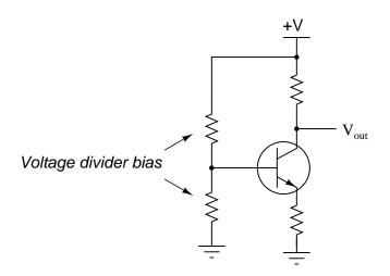
However, if we were to directly connect a source of AC signal voltage to the junction between the two voltage divider resistors, the circuit would most likely function as if there were no voltage divider network in place at all:
