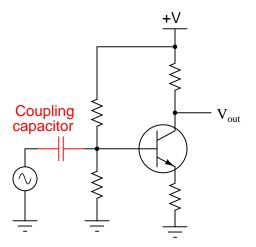
Explain why a coupling capacitor is necessary to allow the voltage divider to work in harmony with the AC signal source. Also, identify what factors would be relevant in deciding the size of this coupling capacitor.
