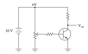
If we were to apply a sinusoidal AC signal to the input of this transistor amplifier circuit, the output would definitely *not* be sinusoidal:
