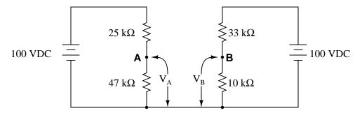
Now, calculate the voltage between points **A** (red lead) and **B** (black lead) ( $V_{AB}$ ). file 01725
