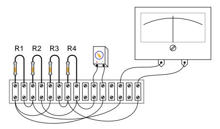
Such a bridge circuit needed to be built with three "standard" resistors, having precisely known resistances. At least one of these resistors needed to be adjustable, with a precision scale attached to it for indication of its resistance at any given position. The source ("excitation") voltage did not not have to be precise, and the null meter only had to be sensitive and accurate at zero volts.
