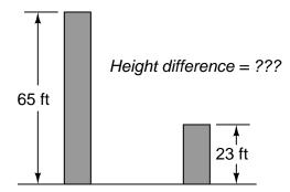
The height of each object is analogous to the voltage dropped across each of the lower resistors in the voltage divider circuits. Like voltage, height is a quantity measured between two points (the top of the object and ground level). Also like the voltage  $V_{AB}$ , the difference in height between the two objects is a measurement taken between two points, and it is also found by subtraction.
