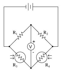
However something has failed in this circuit, because the voltmeter is "pegged" fully negative and will not change with varying light exposures on the two cells. Identify at least two possible failures that could cause the voltmeter to over-range in the negative direction.
