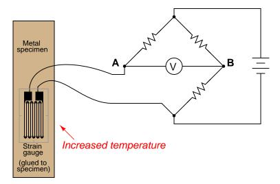
The bridge circuit is supposed to respond to changes in specimen strain, but explain what will happen to the voltage measured across this bridge circuit  $(V_{AB})$  if the specimen's temperature increases (with no stress applied), assuming that the bridge begins in a balanced condition with no strain on the gauge, at room temperature. Assume a positive  $\alpha$  value for the strain gauge conductors.
