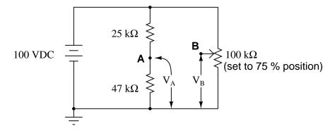
Now, calculate the voltage between points  ${\bf A}$  (red lead) and  ${\bf B}$  (black lead).  $\underline{{\rm file}~00542}$
