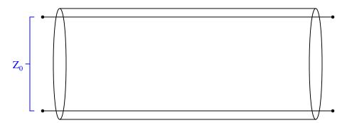
A two-conductor cable of uniform construction will exhibit a uniform characteristic impedance  $(Z_0)$  due to its intrinsic, distributed inductance and capacitance:
