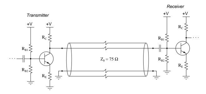
How would we choose the component values in each transistor amplifier circuit to naturally terminate both ends of the 75  $\Omega$  cable?
