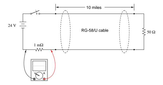
What sort of waveform or pulse would the oscilloscope register after switch closure?  $\underline{\text{file }00132}$
