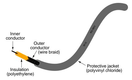
Note the "50 ohm" rating printed on the jacket of the cable. What will an ohmmeter register when connected between the inner conductor and shield of the cable? What will an ohmmeter register when connected between opposite ends of either the inner conductor or the shield, from one end of the cable to the other?
