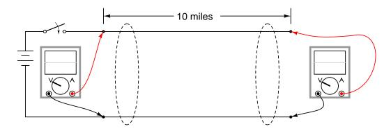
If a battery and switch were connected to one end of a 10-mile long cable, and two oscilloscopes were used to record voltage at either end of the cable, how far apart in time would those two pulses be, assuming a propagation velocity equal to 69% the speed of light (in other words, the cable has a *velocity factor* equal to 0.69)?
