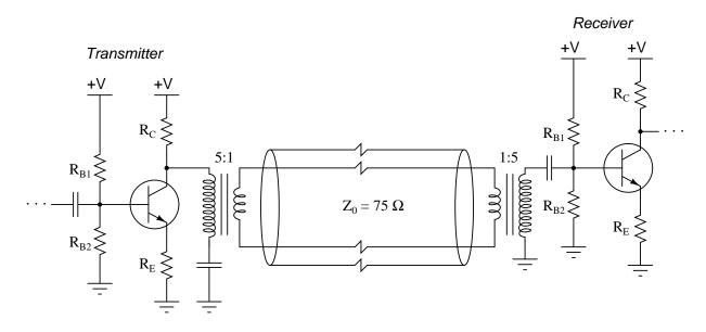
How would we choose the component values in each transistor amplifier circuit to naturally terminate both ends of the 75  $\Omega$  cable?
