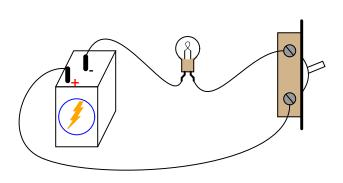
Follow-up question: suppose the circuit were built like this but the light bulb did not turn on when the switch was closed. Identify at least five specific things that could be wrong with the circuit to cause the light not to turn on when it should.
