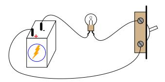
Follow-up question: suppose the circuit were built like this but the light bulb did not turn on when the switch was closed. Identify at least five specific things that could be wrong with the circuit to cause the light not to turn on when it should.
