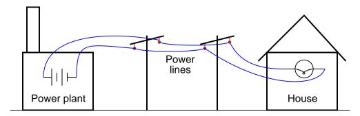
Why would anyone use two wires to conduct electricity from a power plant to a house, as shown, when they could simply use one wire and a pair of *ground* connections, like this?
