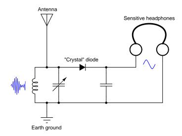
Explain how the AM radio signal becomes "demodulated" into an audio-frequency signal, through the clipping action of the diode.
