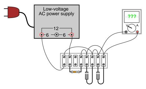
The diodes are model 1N4001, each. The resistor's color code is Brown, Black, Orange, Silver.  $\underline{file~01108}$
