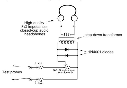
What purpose do the two diodes serve in this circuit? Hint: if you remove the diodes from the circuit, you will not be able to hear the difference in most cases! file 00983
