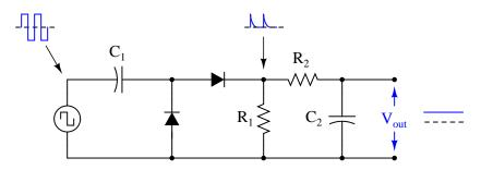
Explain what happens to the output voltage as the input frequency is increased, assuming the input voltage amplitude does not change. Can you think of any practical applications for a circuit such as this?  $\frac{\text{file } 02129}{\text{file } 02129}$
