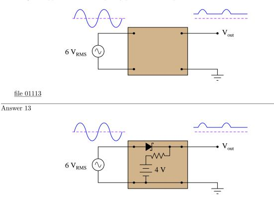
Follow-up question: explain why a *Schottky* diode is shown in this circuit rather than a regular silicon PN-junction diode. What characteristic(s) of Schottky diodes make them well suited for many clipper applications?
