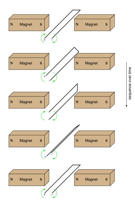
Challenge question: if a resistor were connected between the ends of this wire loop, would it "see" direct current (DC), or alternating current (AC)?
