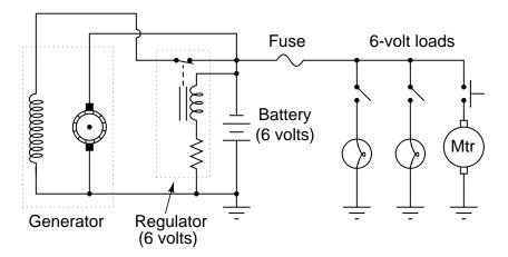
The mechanic's plan is to replace all the 6-volt loads with 12-volt loads, and use two 6-volt batteries connected in series, with the original (6-volt) regulator sensing voltage across only one of those batteries:
