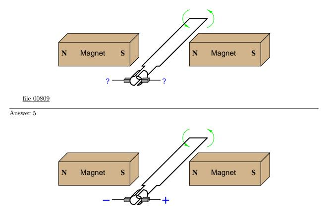
Follow-up question: does the polarity measured at the two carbon brushes ever reverse? Or, to phrase the question another way, if a resistor were connected between the two brush contacts, would it "see" direct current (DC) or alternating current (AC)? Explain your answer.
