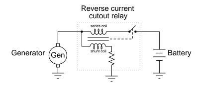
When the generator is spun fast enough, it generates enough voltage to energize the shunt coil with enough current to close the relay contact. This connects the generator with the battery, and charging current flows through the series coil, creating even more magnetic attraction to hold the relay contact closed. If the battery reaches a full charge and does not draw any more charging current from the generator, the relay will still remain closed because the shunt coil is still energized.
