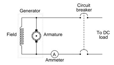
Obviously, there must be some inherent limit to this otherwise vicious cycle. Otherwise, the output voltage of a shunt-wound DC generator would be completely unstable.  $\frac{file\ 00814}{file\ 00814}$
