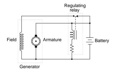
Simple electromechanical relay circuits such as this one were very common in automotive electrical systems during the 1950's, 1960's, and 1970's. The fundamental principle upon which their operation is based is called *negative feedback*: where a system takes action to *oppose* any change in a certain variable. In this case, the variable is generator output voltage. Explain how the relay works to prevent the generator from overcharging the battery with excessive voltage.
