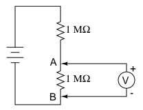
However, if you perform this same experiment using a real voltmeter, the measurement obtained with the meter will be substantially different from what *should* be there, based on a prediction of  $\frac{1}{2}E_{battery}$ . Explain why the voltmeter registers as it does. What is it about this circuit that causes the measurement to be so far off from the prediction, when we know full well that other voltage divider circuits we've constructed do not exhibit any significant error?
