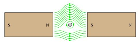
This interaction of magnetic flux lines (the bar magnets' straight lines versus the wire's circles) will produce a mechanical force on the wire (called the *Lorentz* force). Which direction will this force act? Also, determine the direction of current through the conductor (seen from an end-view in the above illustration) necessary to produce the circular magnetic flux shown.
