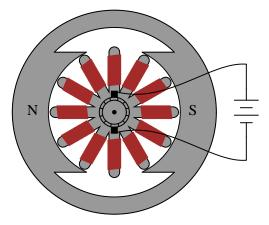
This particular motor is of the "permanent magnet" type, with wire windings only on the armature. Write the necessary magnetic polarities ("N" for north and "S" for south) on the armature's electromagnet pole tips, in order to sustain a *clockwise* rotation.
