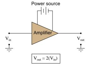
If we were to try to rate this amplifier's gain in terms of the relative *power* dissipated by a given load resistance ( $P_{load}$  when powered by  $V_{out}$ , versus  $P_{load}$  when powered by  $V_{in}$ ), what ratio would we calculate? In other words, what is the ratio of power for a given load resistance, when powered by a given voltage, versus when powered by a voltage that is twice as much?
