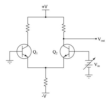
Would you characterize this transistor amplifier as being *inverting* or *noninverting*, with the base terminal of transistor Q1 being considered the input? Explain your answer.
