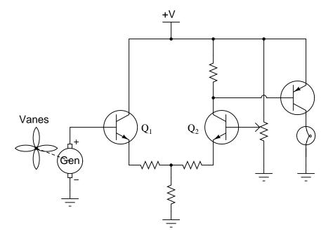
Based on your understanding of differential pair circuits, is this a high-speed wind indicating circuit or a low-speed wind indicating circuit?
