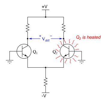
Follow-up question: what does this phenomenon mean with regard to the stability of differential-pair transistor circuits under different operating conditions? What might be a good way to maximize circuit stability over a wide range of operating temperatures?
