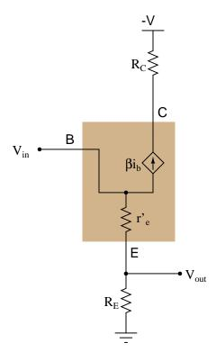
Follow-up question: the voltage gain equation for this type of transistor amplifier is usually shown in a simpler form that what I provided at the end of the question. Write this simpler form, and explain why it is approximately true.
