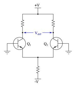
What would happen to this differential voltage  $(V_{diff})$  if transistor Q2 were to increase in temperature, while transistor Q1 remained at the same temperature? Explain your answer. file 00887
