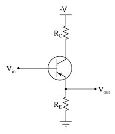
Also, explain how to derive the voltage gain equation for this amplifier:
