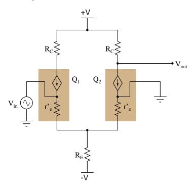
Write an approximate equation describing the differential voltage gain for a differential pair circuit such as this, in terms of the component values:
