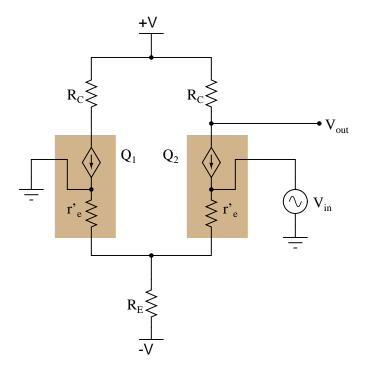
Here, a differential pair circuit is driven by an input voltage at the base of  $Q_1$ , while the output is taken at the collector of  $Q_2$ . Meanwhile, the other input  $(Q_2 \text{ base})$  is connected to ground:
