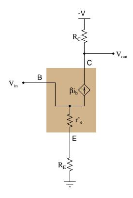
Follow-up question: the voltage gain equation for this type of transistor amplifier is usually shown in a simpler form that what I provided at the end of the question. Write this simpler form, and explain why it is approximately true.
