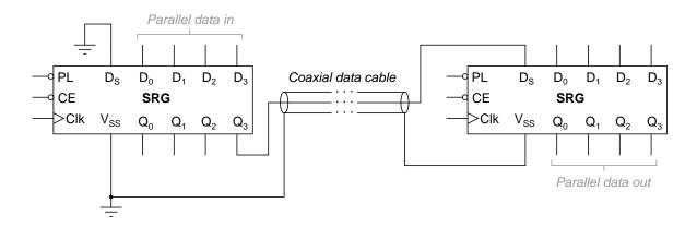
Specify what logic states would have to be input at the PL, CE, and Clk terminals of each shift register, and at what times, to successfully load four bits of parallel data, shift them serially over the coaxial data cable, and then hold them at the outputs (Q) of the receiving shift register. file 02997
