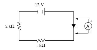
Usually, ammeters are connected in *series* with the component whose current is to be measured. However, in this case a parallel connection is acceptable. Explain why, and determine the ammeter's current reading in this circuit.
