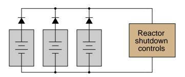
Challenge question: it would be nice if there were indicator lamps in the system to warn maintenance personnel of a shorted power supply. Is there any way you can think of to place light bulbs in this system somewhere, so that one will light up in the event of a power supply failure?
