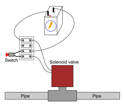
The only problem with this simple circuit is that the switch contacts suffer from extensive arcing caused each time the solenoid is de-energized. One way to combat this arcing, though, is to connect an ordinary rectifying diode in parallel with the solenoid like this:
