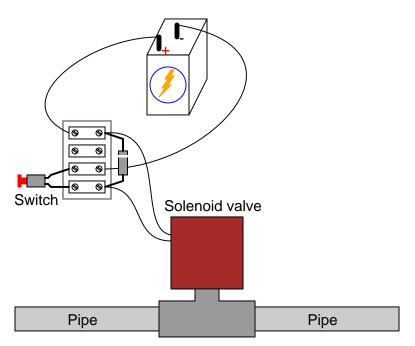
With a diode in place, the release time for the solenoid increases measurably. In other words, it takes longer for the solenoid to completely de-magnetize after the switch contacts open, than if there is no diode in the circuit.
