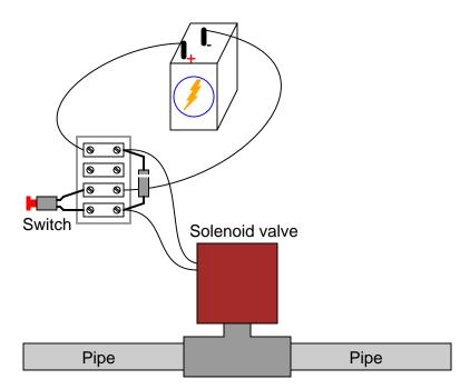
Explain what causes the excessive arcing at the switch contacts, and how the presence of a diode in the circuit completely eliminates it.
