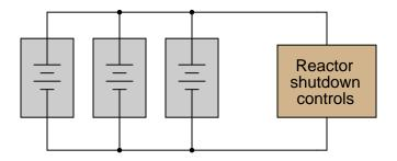
The only problem with this scenario is the possibility of one of these power sources internally shortcircuiting. Describe what would happen if one of the three DC power sources developed an internal shortcircuit, and explain how this problem could be avoided by placing diodes in the circuit.  $\frac{file\ 00985}{file\ 00985}$
