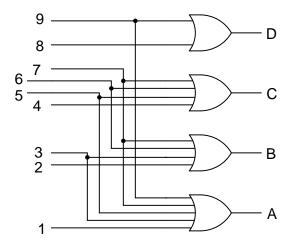
Also, determine which output (D or A) is the  $most\ significant\ bit$  of the BCD output.  $\underline{file\ 03003}$
