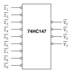
Describe what sort of input conditions would be required to make it generate the code for the number 7, and how that numerical quantity would be represented on the output (Y) lines.
