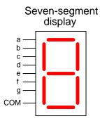
A special decoder circuit is needed to translate 4-bit BCD codes into the particular combinations of segment activations that represent decimal digits.
