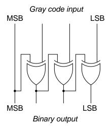
Challenge question: this circuit is not as suited to high-speed conversion as a binary-to-Gray converter, even though it uses the same quantity and same type of logic gate. Explain why problems may arise if this circuit is forced to convert Gray code inputs that are changing rapidly (for instance, translating the output of a Gray-code rotary encoder into binary, when the mechanical encoder is rotating at a very high speed).
