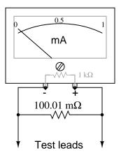
A power dissipation rating of at least 10 watts is necessary for this application.
