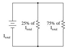
Hint: one resistor carries three times the current of the other.  $\underline{file \ 01428}$
