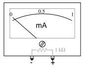
Show how a single resistor could be connected to this ammeter to extend its range to 0 to 10 amps. Calculate the resistance of this "range" resistor, as well as its necessary power dissipation rating.
