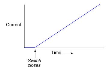
Challenge question: real wire coils contain electrical resistance (unless they're made of superconducting wire, of course), and we know how voltage equilibrium occurs in resistive circuits: the current converges at a value necessary for the resistance to drop an equal amount of voltage as the source. Describe, then, what the current does in a circuit with a *real* wire coil, not a superconducting wire coil.
