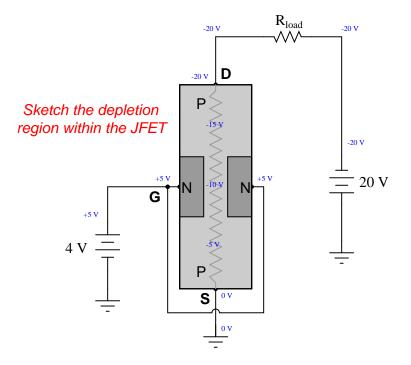
Something *really* interesting happens if we reverse the polarity of the 20 volt source: the relationship between drain and source changes, and so does the depletion region profile. Sketch the new varying width of the depletion region with the 20 volt source reversed, and comment on what you see:
