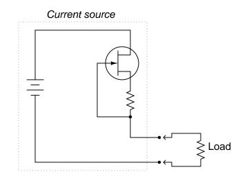
The resistor creates a voltage drop that tries to pinch off the JFET as current increases. To put it in colloquial terms, "when the current *zigs*, the JFET *zags*."
