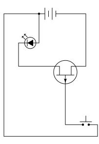
In each case, the load de-energizes with switch closure, and energizes when the switch is opened.
