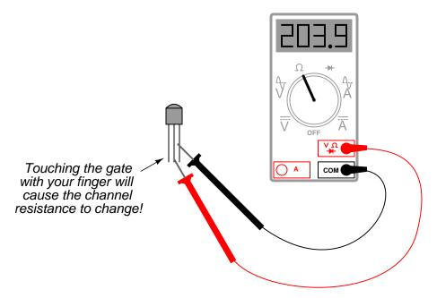
Such a degree of sensitivity is unheard of in bipolar junction transistors. Explain why the JFET is so sensitive, and comment on what advantages and disadvantages this gives the JFET as an electronic device. <u>file 02062</u>
