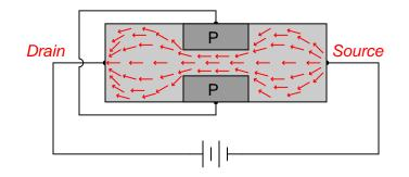
This makes the right-hand terminal the source and the left-hand terminal the drain.
