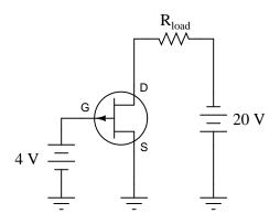
If we connect a gate-to-source voltage  $(V_{GS})$  large enough to force the transistor into cutoff mode, the JFET channel will act as a huge resistance. If we look carefully at the voltages measured with reference to ground, we will see that the width of the depletion region must vary within the JFET's channel. Sketch this varying width, given the voltages shown in the illustration:
