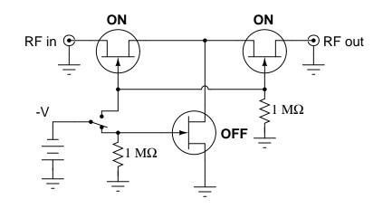
With the switch in the position shown, the circuit will pass the RF signal from input to output.
