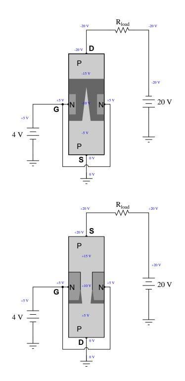
Follow-up question: you can see that the transistor doesn't even cut off as expected with the 20 volt source reversed. What would we have to do to get this JFET to cut off with a only 4 volt control signal, since having reversed the 20 volt source?
