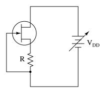
Despite wide variations in  $V_{DD}$ , the current in this circuit will remain relatively constant. The reason this circuit works as it does is *negative feedback*. Explain what causes negative feedback to occur in this circuit, and why it has a stabilizing effect on the current.
