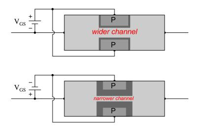
Follow-up question: why do you suppose this type of transistor is called a *field-effect* transistor? What "field" is being referred to in the operation of this device?
