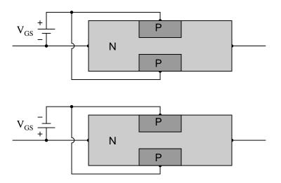
Note how the different depletion region sizes affect the conductivity of the transistor's channel.  $\underline{file \ 02055}$
