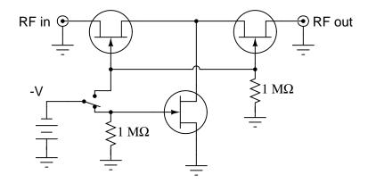
Identify the "on" and "off" states of the three JFETs in this circuit with the switch in the position shown in the schematic, and also determine whether the switch position shown in the diagram is for "passing" or "blocking" the RF signal from input to output.
