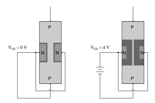
Something not immediately apparent about this effect is that the formation of a wide depletion region necessary for cut-off of a field-effect transistor is *also* affected by the drain-to-source voltage drop  $(V_{DS})$ .
