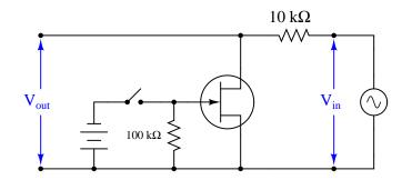
What effect will opening and closing the toggle switch have on the AC signal measured at the output terminals?
