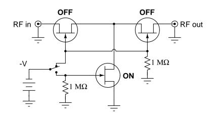
With the switch in the position shown, the circuit will *block* the RF signal from getting to the output.
