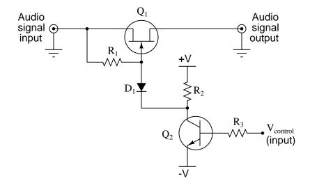
What sort of signal is necessary at pin  $V_{control}$  to allow the audio signal to pass through the JFET, and what sort of signal turns the JFET off? Also, explain the purpose of each of these components in the audio switching circuit:
