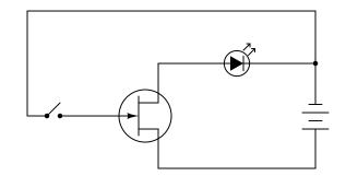
Explain what is happening here, and also propose a solution to eliminate the unpredictability when the switch is open.
