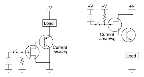
Determine for each circuit whether the load becomes energized when the switch is *closed* or when it is *opened*, and explain how each one works.
