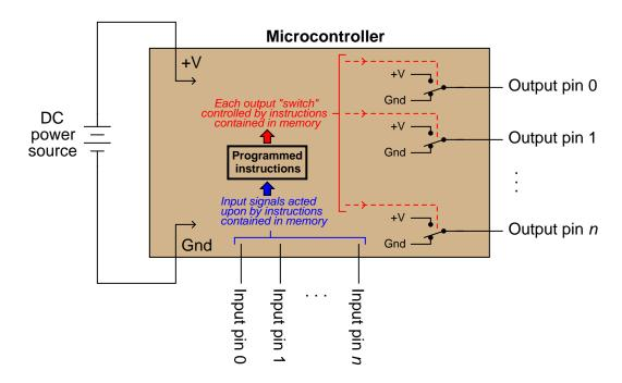
Microcontrollers may be programmed to emulate the functions of digital logic gates (AND, OR, NAND, NOR, etc.) in addition to a wide variety of combinational and multivibrator functions. The only real limits to what a microcontroller can do are memory (how large of a program may be stored) and input/output pins on the MCU chip.
